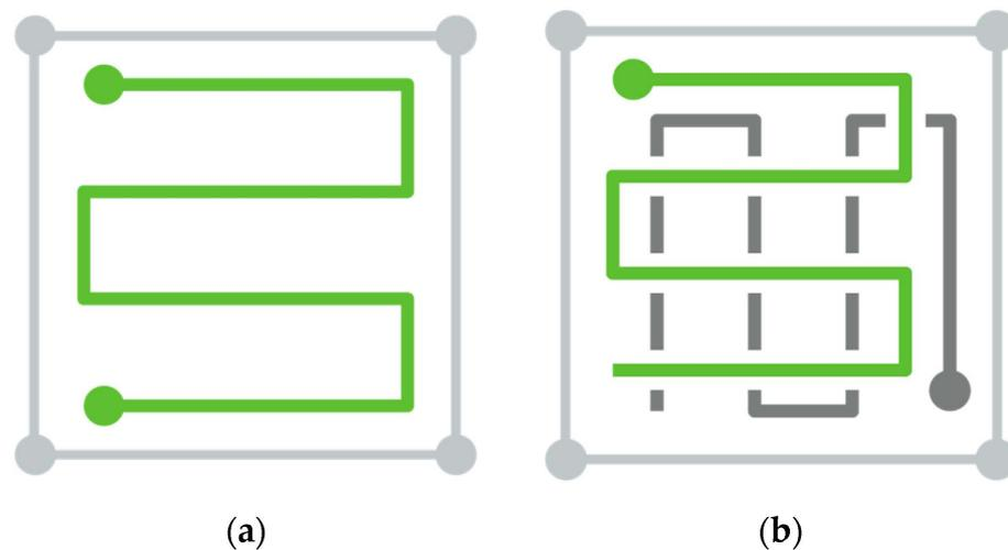
**Figure 2.** (a) Depiction of a single-grid flight pattern; (b) depiction of a double-grid flight pattern.
