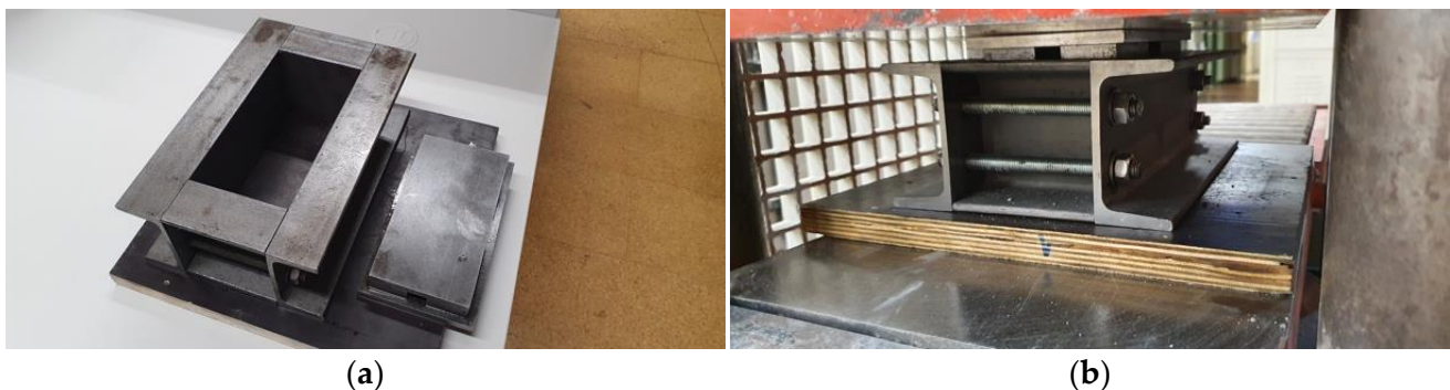
Figure 2. Mould used (a) before filling and (b) filled and under compaction.
