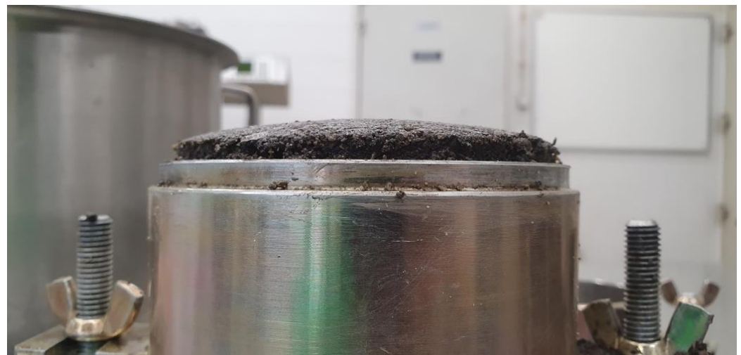
Figure 6. Visible volume expansion of MIBA seconds after compaction to the mould's top surface level.
