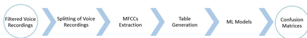
**Figure 1.** Classification process pipeline: the voice recordings have been split into windows of 30 s. Then, informative features have been extracted and used as input for the ML framework.
