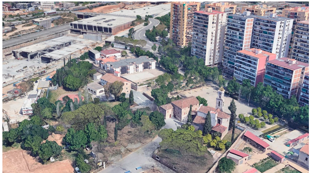
Figure 11. The railway tunnel entrances for the Sagrera complex in construction. The church in front of the apartment blocks remains. The old Puente de Trabajo has been replaced by a new bridge, requiring the swerve in the road around the tunnel entrance construction (source: Google Earth).
