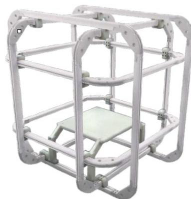
**Figure 2.** View of the three-axis Helmholtz coil system. In its center, the homogenous induced magnetic field covers a volume of around  $25 \times 25 \times 25 \text{ cm}^3$ . The system is controlled with a desktop, which manages each field axis in terms of shape, frequency, and amplitude, independently.
