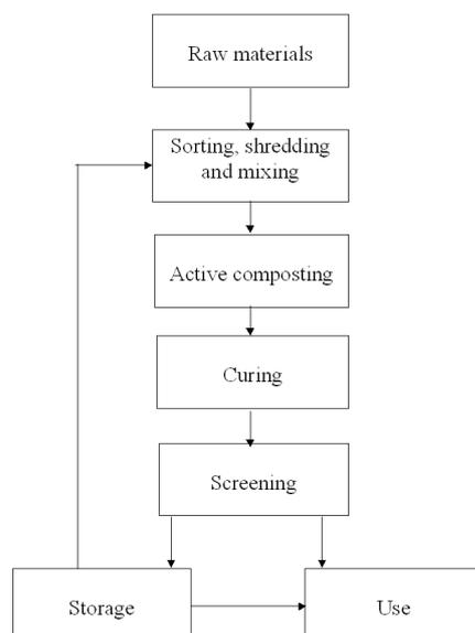
**Figure 1.** Flow chart of a typical composting process.
