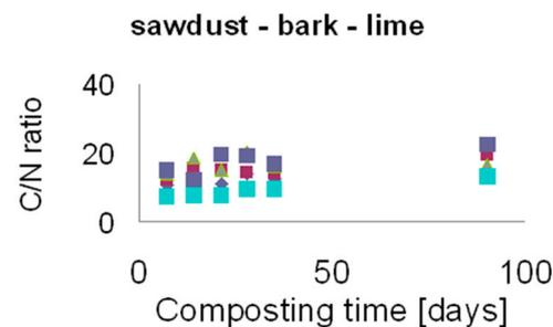
Figure 3. Relationships between C/N ratio and time of composting raw and limed sewage sludge.
