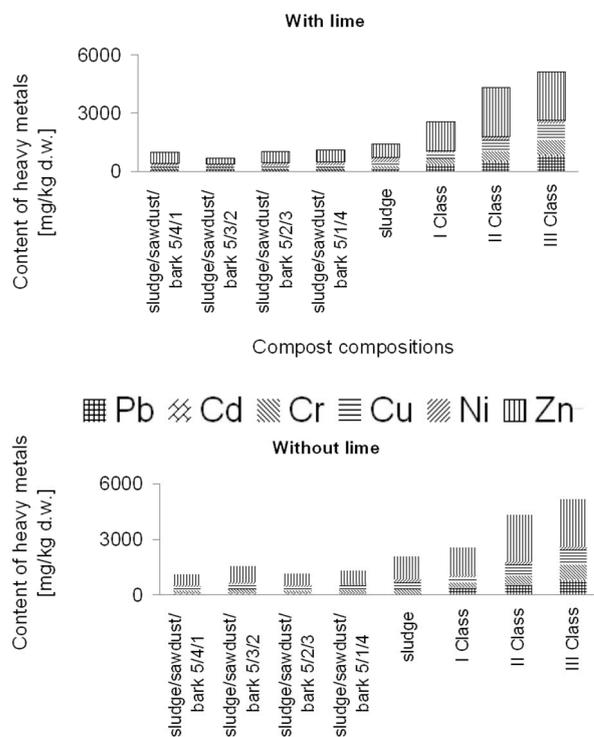
Figure 4. Content of heavy metals in composts of raw and limed sewage sludge.
