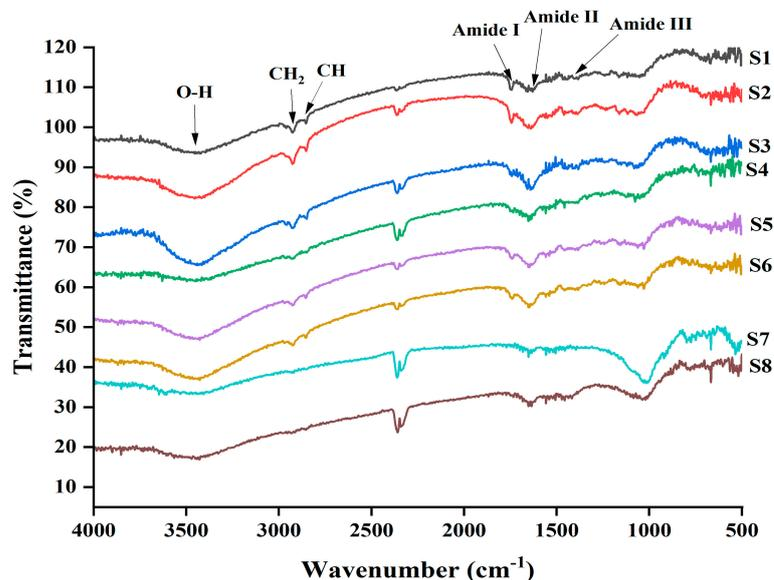
**Figure 3.** FT-IR analysis of different edible paper sheets produced from *A. philoxeroides* and *H. molitrix*. S1: Ap300/Hm100 (Boil); S2: Ap300/Hm100 (Boil); S3: Ap200/Hm200 (Boil); S4: Ap100/Hm300 (Boil); S5: Ap400/Hm0 (Non-Boil); S6: Ap300/Hm100 (Non-Boil); S7: Ap200/Hm200 (Non-Boil); and S8: Ap100/Hm300 (Non-Boil).
