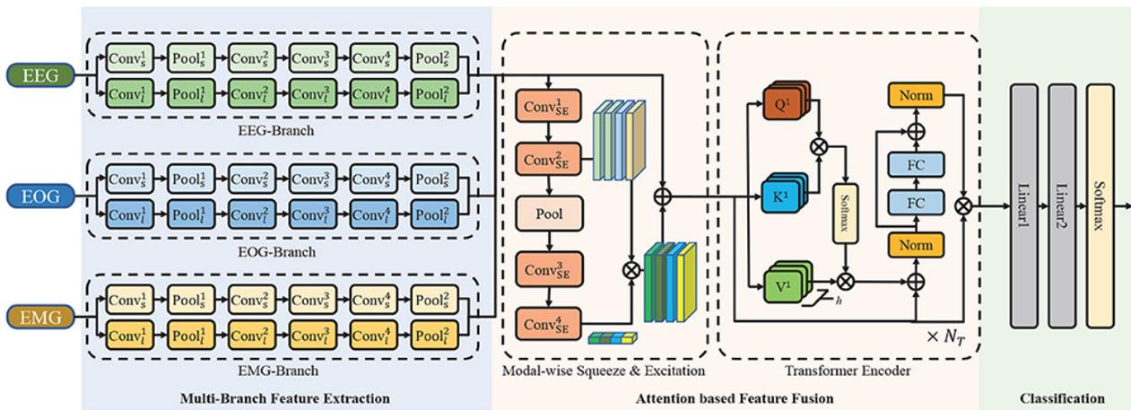
Figure 11. Model architecture for MMASleepNet. Image taken from [168].
