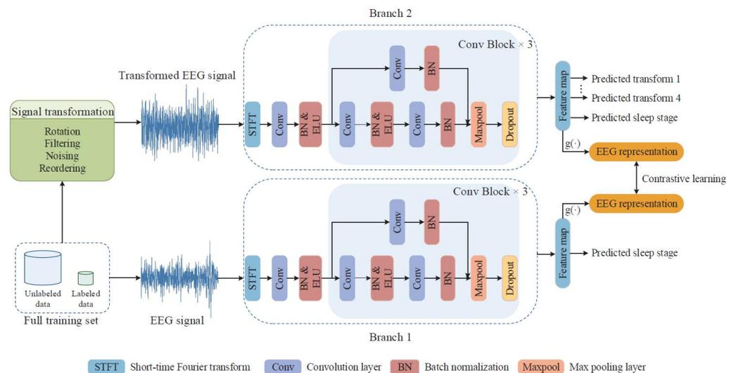
Figure 15. Model architecture for MtCLSS. Image taken from [175].
