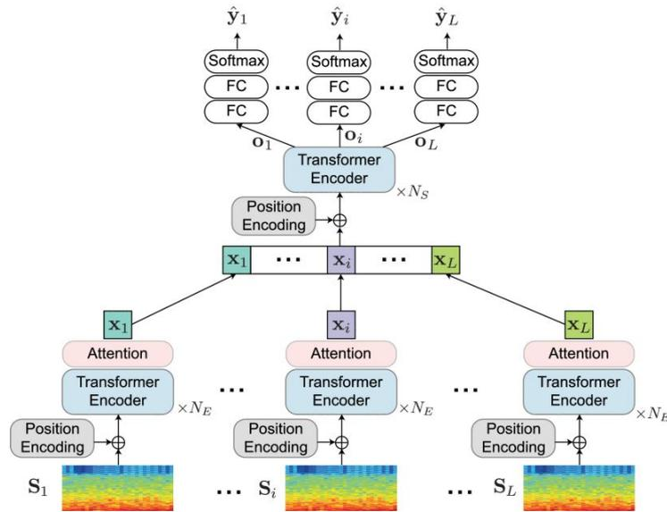
Figure 9. Model architecture for SleepTransformer. Image taken from [166].
