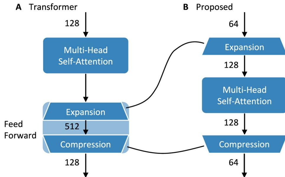
**Figure 13.** Difference between transformer and ENGELBERT. Image taken from [170].
