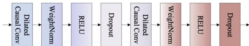
Figure 6. Temporal convolution network. Image taken from [85].
