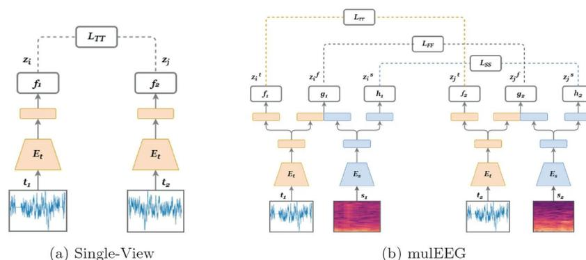
Figure 19. Model architecture for mulEEG. Image taken from [56].
