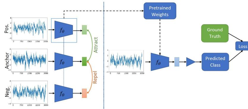
Figure 17. Model framework for SCL-SSC [178]. Image taken from [178].
