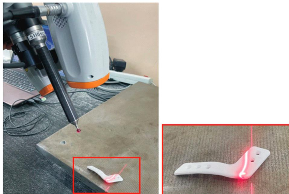
**Figure 8.** The process of measuring the geometry of a prototype surgical plate.
