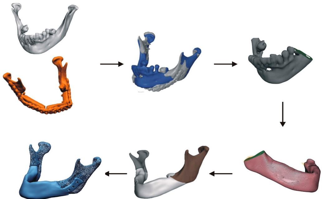
**Figure 4.** CAD modeling process of the prototype implant of the anterior part of the mandible.
