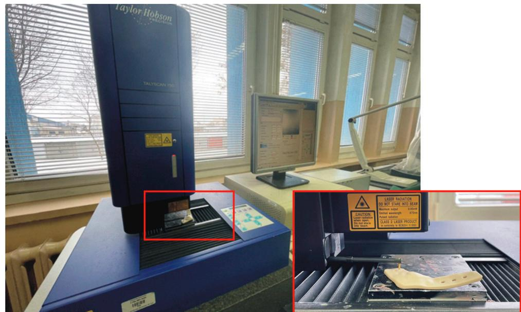
**Figure 9.** The process of measuring the surface topography of a manufactured surgical plate.
