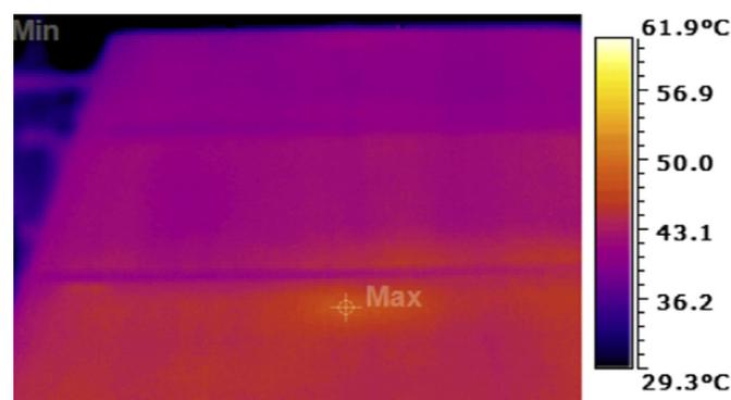
**Figure 9.** Infrared imaging to discover high-temperature cells in a PV module [18].
