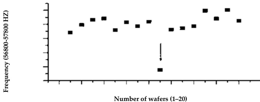
**Figure 11.** Ultrasonic inspection of several cell wafers showing cell no. 11 has an abnormal reduction in frequency, indicating a crack failure [197].
