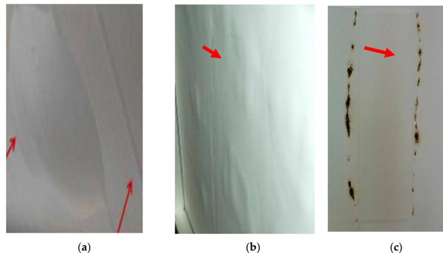
**Figure 7.** (a) Backsheet bubbles [130]. (b) Backsheet delamination [130]. (c) Burn marks caused by a hotspot in the backsheet [138].
