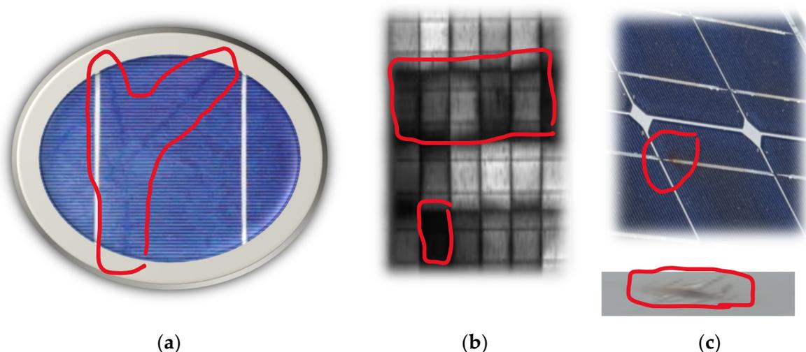
**Figure 6.** (a) PV module affected by snail track failure [127]. (b) PID failure detected by electroluminescence image [137]. (c) Hotspot burned the cell solder bonding and exhibited burn marks on the backsheet [138].
