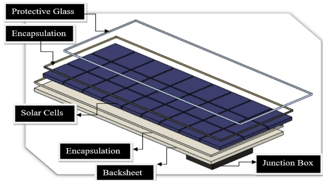
**Figure 3.** PV module components designed using Fusion 360 software. (The software is from Autodesk and is called Fusion 360. The version is 2.0 and Autodesk are located in San Francisco, CA, USA).
