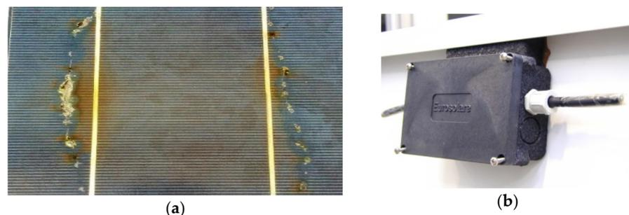
**Figure 8.** (a) Failed bypass diodes leading to hotspots [138]. (b) Poor bonding of J-box [137].
