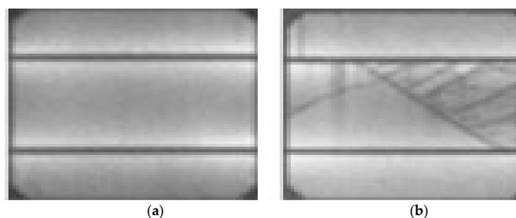
**Figure 10.** (a) EL imaging of a healthy monocrystalline solar cell. (b) EL imaging of a cracked monocrystalline solar cell [196].
