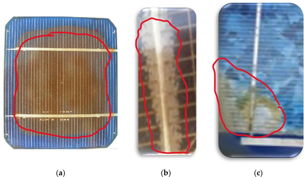
**Figure 5.** (a) Brown discolouration of PV cell [108]. (b) PV module affected by delamination [66]. (c) PV module affected by delamination that led to corrosion [109].
