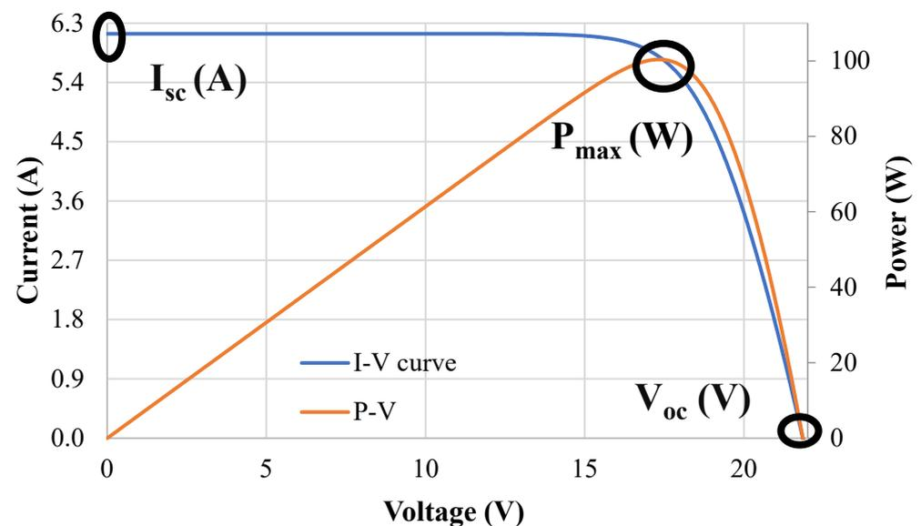
**Figure 12.** Current–voltage and power–voltage curves display the major parameters of a solar cell;  $I_{sc}$ , current at zero volts;  $V_{oc}$ , voltage at zero amps; and  $P_{max}$ , maximum power output. The circles show the location of short circuit current, open circuit voltage and maximum power point.
