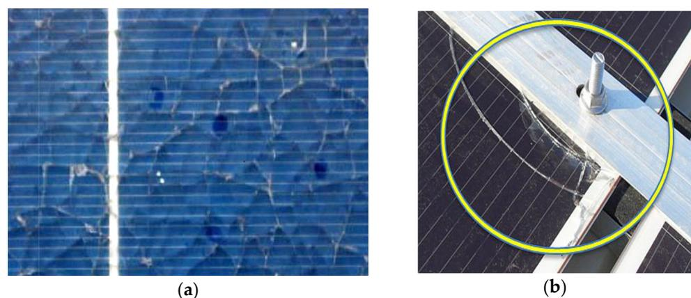
**Figure 4.** (a) Example of PV module with shattered protective glass [74]. (b) Broken glass due to installation fault by over-tightening a bolt [15].
