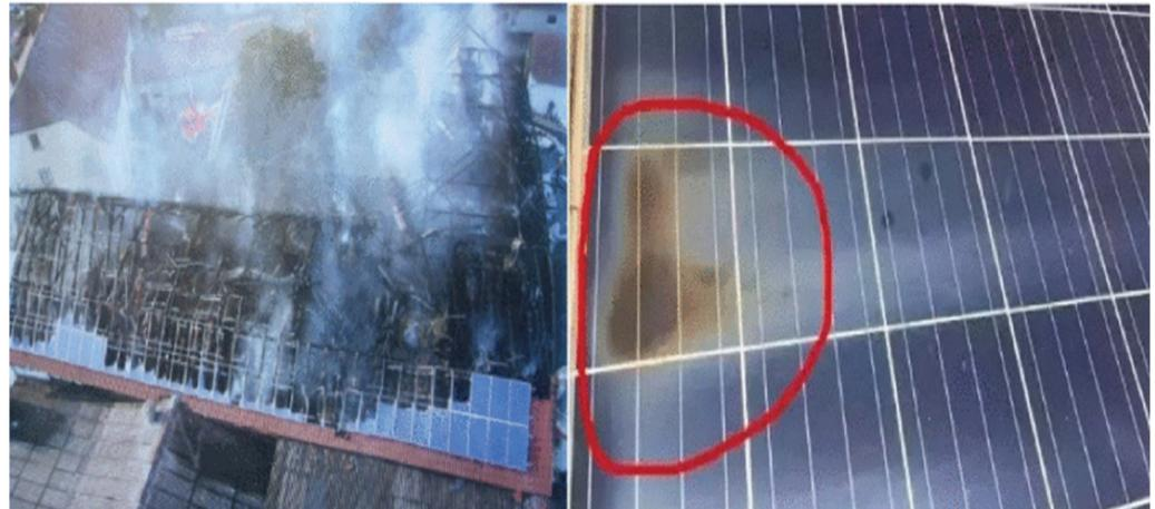
**Figure 2.** Fire incident in PV array initiated by hotspot failure [45].
