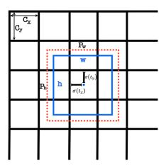
**Figure 2.** Prediction of bounding box. YOLOv7 will predict the width and height of the box as offsets from cluster centroids and center coordinates of the box relative to the location of the filter application using a sigmoid function. The red dotted indicates the prior anchor, and the blue square is the prediction.
