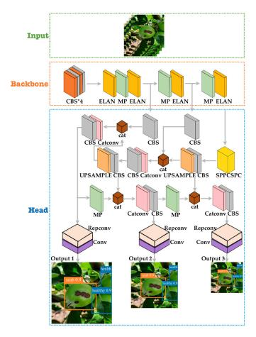
**Figure 4.** An overview of the proposed model of  $\mathbb{CARAFE}$  architecture incorporated in YOLOv7 network architecture.
