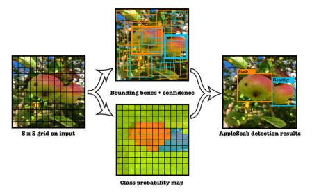
**Figure 1.** YOLO model detection. The classification task is addressed while dealing with regression. Therefore, each interested class (Healthy, Scab) is represented under different colors to illustrate the YOLO detection model.
