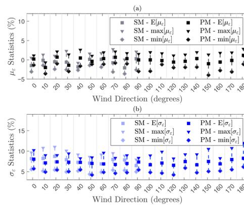
**Figure 8.** (a) mean errors in the variance for SM and PM layouts, and (b) standard deviation of the errors in the variance for the SM and PM layouts.
