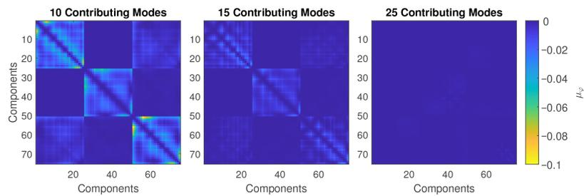
**Figure 19.** Mean error in the correlation coefficients, considering 10, 15, and 25 modes, for SM layout and wind direction  $\beta = 0^\circ$ .
