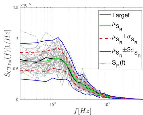
**Figure 6.** Comparison between smoothed PSDs of short-duration records,  $S_R(f)$ , and target PSD of  $CT_{z,20}(t)$  at the 20th floor and wind direction of  $\beta = 0^\circ$ .
