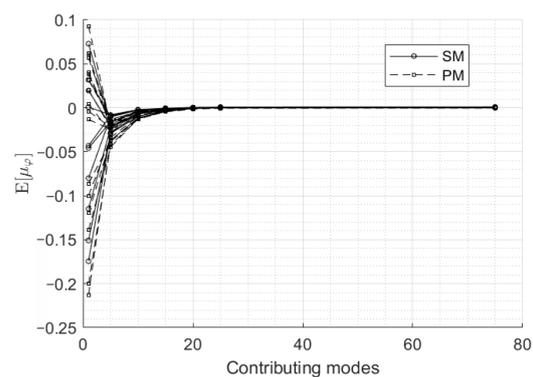
**Figure 22.** Expected difference in the correlation coefficients from the truncation of modes for all wind directions and the SM and PM setups, considering 1, 5, 10, 15, 20, 25, and 75 contributing modes.
