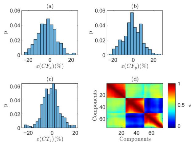
**Figure 13.** Histograms of  $\varepsilon$  associated with SM layout and  $\beta = 0^\circ$  of (a)  $CF_x$ , (b)  $CF_y$ , (c)  $CT_z$ , and (d) correlation coefficients between the components of  $\varepsilon$ .
