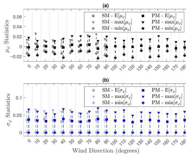
**Figure 12.** (a) mean errors in the correlation coefficients for SM and PM layouts, and (b) standard deviation of the errors in the correlation coefficients for the SM and PM layouts.
