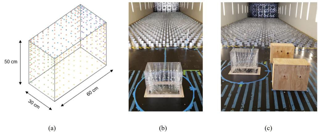
**Figure 1.** (a) illustration of the building model used in the wind tunnel tests, and configuration of the pressure taps, (b) wind tunnel testing with SM setup, and (c) wind tunnel testing with PM setup.
