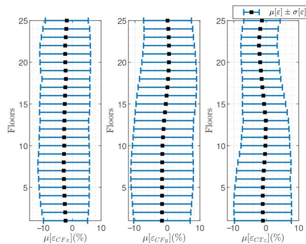
**Figure 7.** Mean error in the variance,  $\mu_\epsilon$ , with standard deviation,  $\sigma_\epsilon$ , for each floor, for the SM layout and  $\beta = 0^\circ$ .
