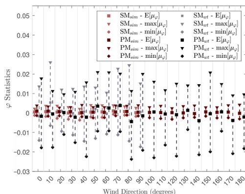
**Figure 17.** Comparison of the difference between the correlation coefficients due to the use of a single smoothed short-duration wind tunnel record (wt) and the simulation model (sim).
