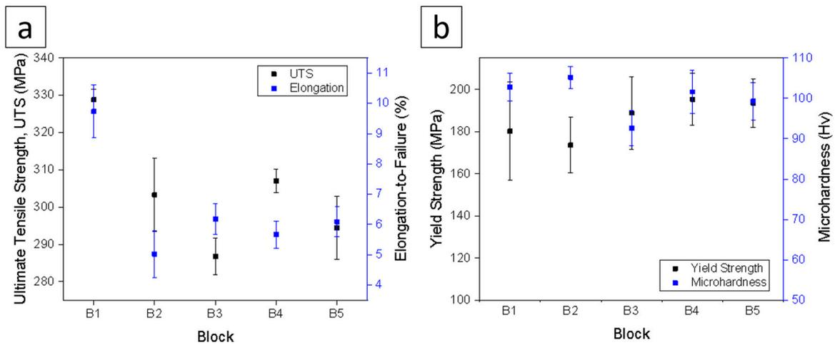
**Figure 9.** Mechanical properties (tested in tension) of the deposited blocks for each cycle: (a) ultimate tensile strength (UTS) and elongation-to-failure and (b) yield strength and microhardness. The error bars correspond to the maximum and minimum measured values.
