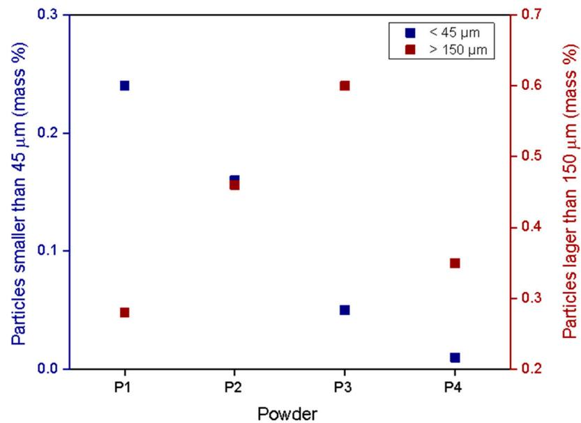
**Figure 5.** The mass percent values of particles smaller than 45 μm and larger than 150 μm after each reuse cycle. The mass percent of powders that fall within the desired 45–150 μm range after each reuse cycle is  $\geq 99\%$ .
