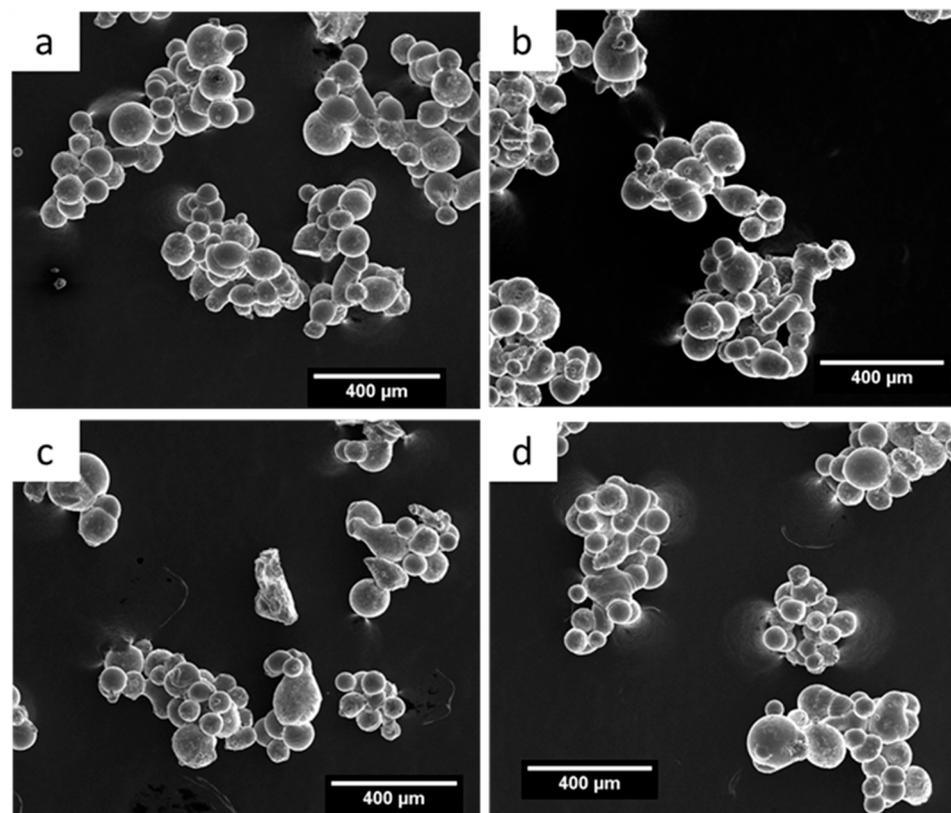
**Figure 6.** SEM micrographs displaying the morphology of the particles larger than 150 μm from powders (a) P1, (b) P2, (c) P3, and (d) P4.
