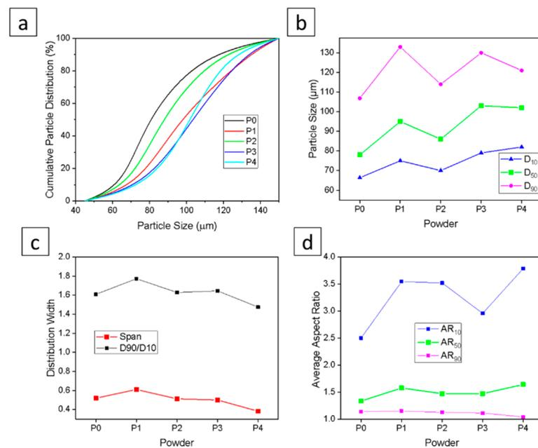
**Figure 4.** (a) Cumulative particle size distributions; (b)  $D_{10}$ ,  $D_{50}$ , and  $D_{90}$ ; (c) distribution width (Span and  $D_{90}/D_{10}$ ); and (d) aspect ratio ( $AR_{10}$ ,  $AR_{50}$ ,  $AR_{90}$ ) for the powders from each reuse cycle.
