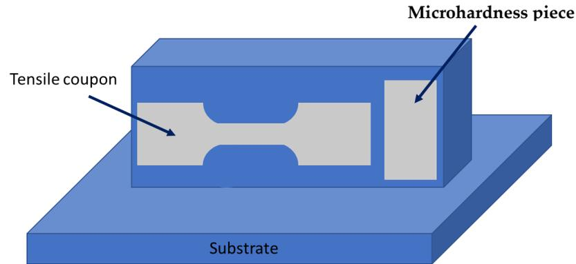
**Figure 2.** Schematic of a deposited block showing the geometry and locations of the dog bone tensile coupons and microhardness piece used for bulk analysis in this study. The dog bone samples have a gauge length of 10 mm and a thickness of 1 mm.
