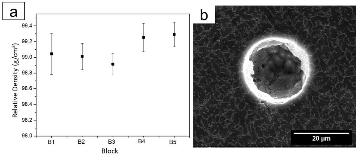
**Figure 8.** (a) The density of deposited blocks for each cycle. The error bars depict the minimum and maximum measured values. (b) Representative micrograph of a pore observed in a deposited block sample.
