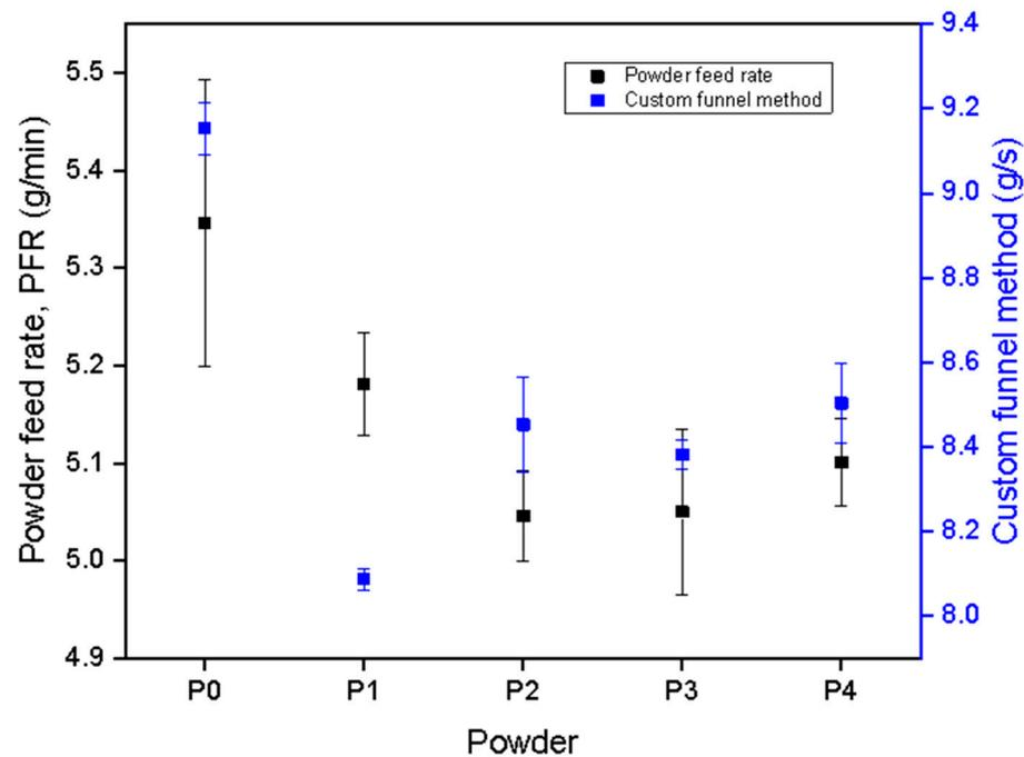
**Figure 7.** Flow rate of the powders from each reuse cycle, measured using the custom-built funnel method and the powder feed rate (PFR) method. The error bars denote the minimum and maximum measured flow rate values.
