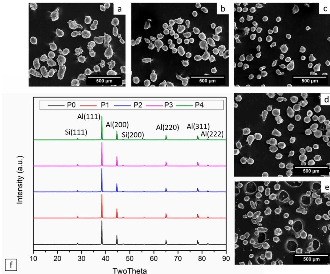
**Figure 3.** SEM micrographs displaying the morphology of the (a) P0, (b) P1, (c) P2, (d) P3, and (e) P4 powders. (f) XRD patterns of the powders from each reuse cycle.
