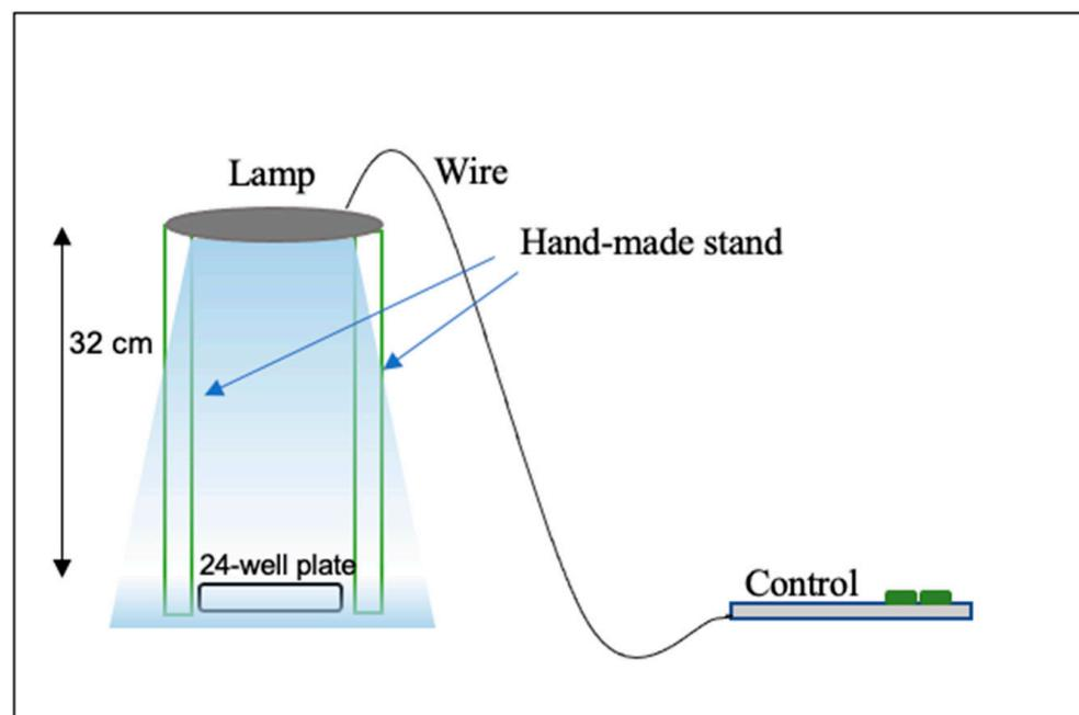
**Figure 2.** The equipment setup (not drawn to scale). The control panel features two green buttons for activating the UVA and UVC switches. The lamp was positioned 32 cm away from a plate with infected cells [13].
