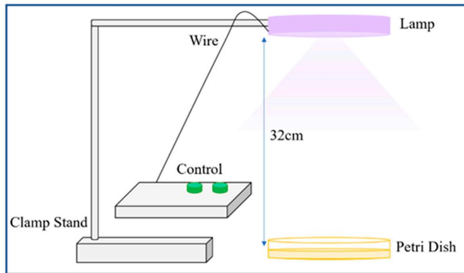
**Figure 1.** The equipment setup (not drawn to scale). The equipment is contained within a blue housing unit that is situated inside a lightbox. The control panel features two green buttons for activating the UVA and UVC switches. The lamp was positioned 32 cm away from the Petri dish [12].
