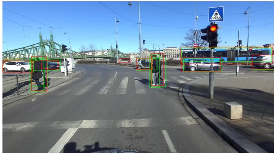
**Figure 3.** Example image of the output of the ZED 2 object detector generated using the toolkit proposed by Padilla et al. [31]. Bounding boxes of the detections are shown in red. Bounding boxes of the ground truth annotations are shown in green.
