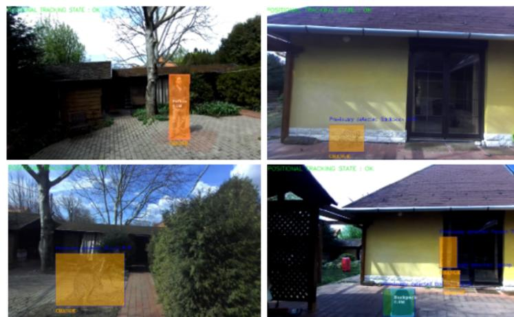
**Figure 7.** Examples of changes due to removed or added objects (shown in orange overlay). For changes caused by removed objects, the point clouds of previous detections are overlaid on the 2D image (top right, bottom left and bottom right example).
