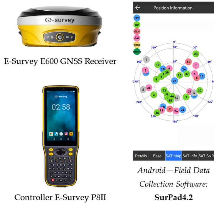
Figure 3. Measurement equipment.
