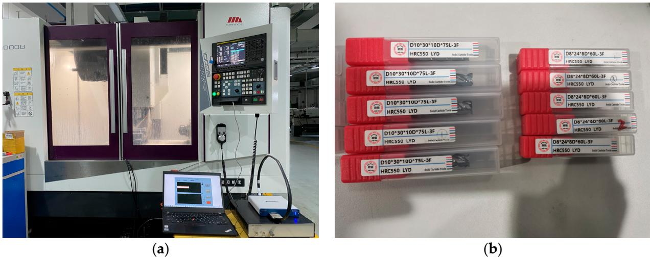
**Figure 9.** Experimental setup and tool selection: (a) CNC machine tool experimental platform; (b) HRC550 LYD hard alloy knife.
