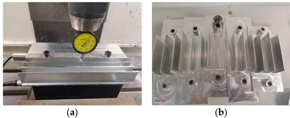
**Figure 12.** All machined parts processed in the experiment: (a) measurement with a dial gauge micrometer; (b) experimental processing of thin-walled specimens.
