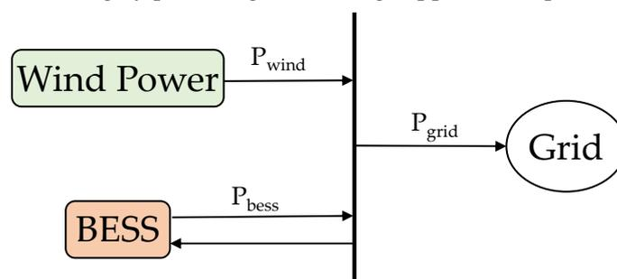
Figure 1. Wind-generated power smoothing scheme.
