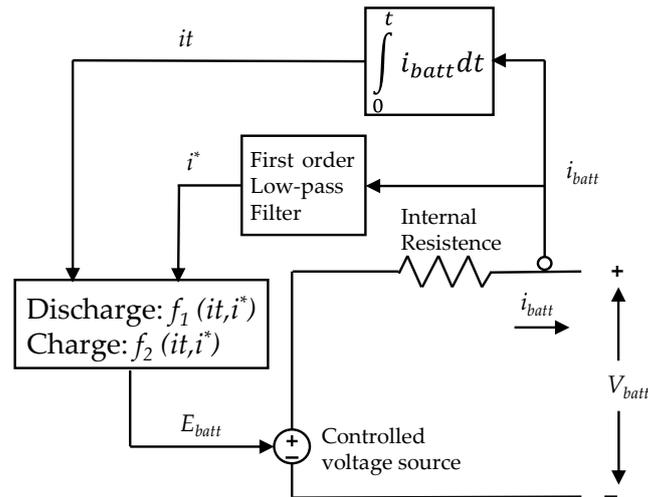
Figure 6. Li-ion battery model simplified schematic diagram.
