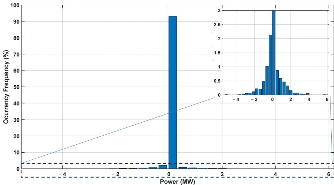
Figure 11. Error between smoothed wind power by fuzzy controller and ideal smoothed wind power.
