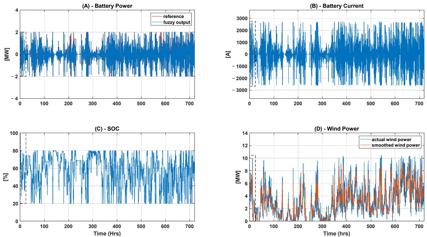
**Figure 10.** Simulation results for 100% initial SOC for one month. (A) Battery Power; dashed line highlight refers to Figure 9A, (B) Battery Current; dashed line highlight refers to Figure 9B, (C) SOC; dashed line highlight refers to Figure 9C, (D) Smoothed wind power; dashed line highlight refers to Figure 9D.
