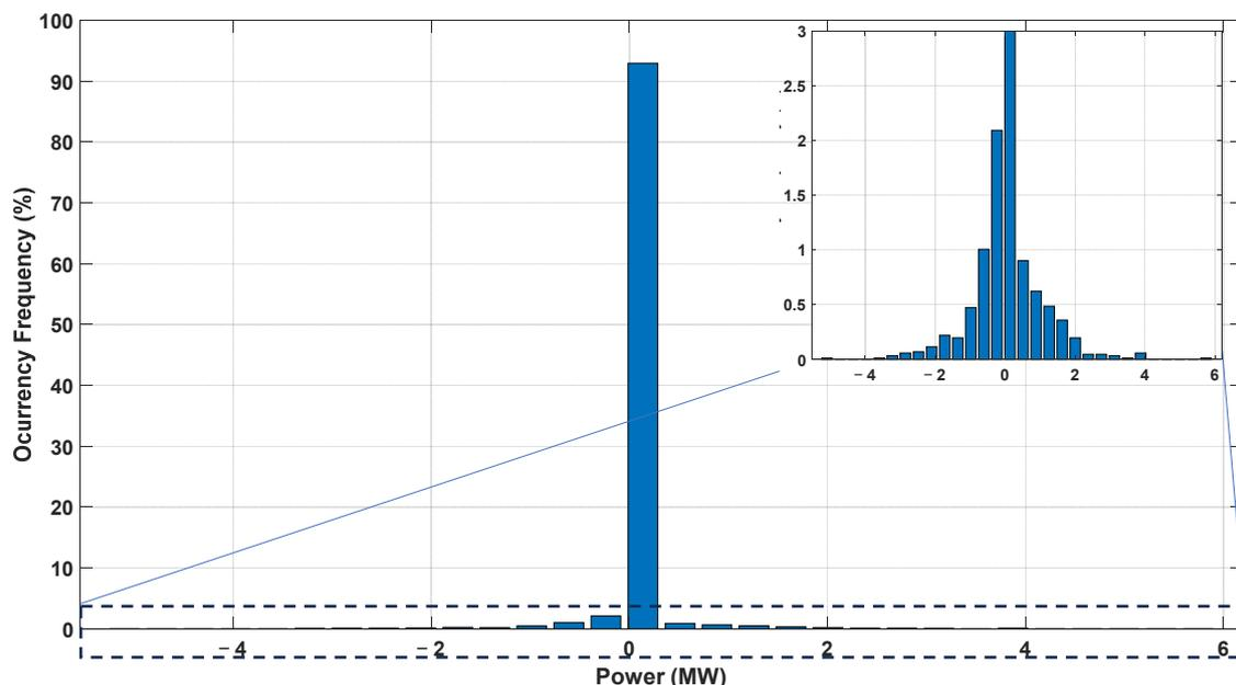
**Figure 15.** Error between smoothed wind power by fuzzy controller and ideal smoothed wind power for initial SOC 10%.
