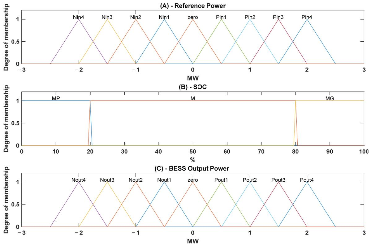
**Figure 8.** Membership functions: (A) reference power; (B) SOC; (C) BESS output power.
