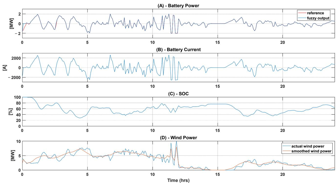
**Figure 9.** Simulation results for 100% initial SOC for the first 24 h. (A) Battery Power, (B) Battery Current, (C) SOC, (D) Smoothed Wind Power.
