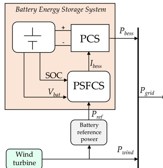
Figure 3. Structure of the Proposed Dispatch Control Strategy based on fuzzy logic.
