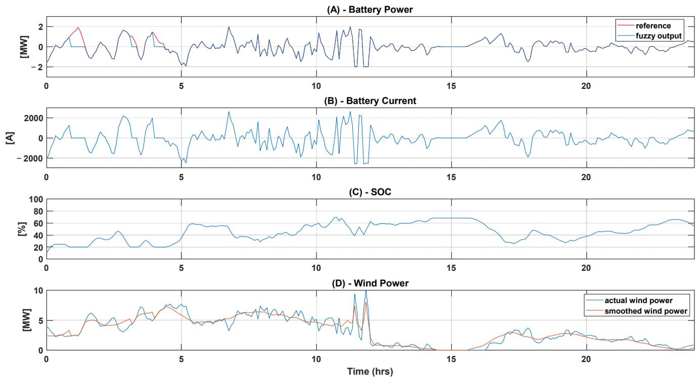
Figure 13. Simulation results for 10% initial SOC for the first 24 h. (A) Battery Power, (B) Battery Current, (C) SOC, (D) Smoothed wind power.
