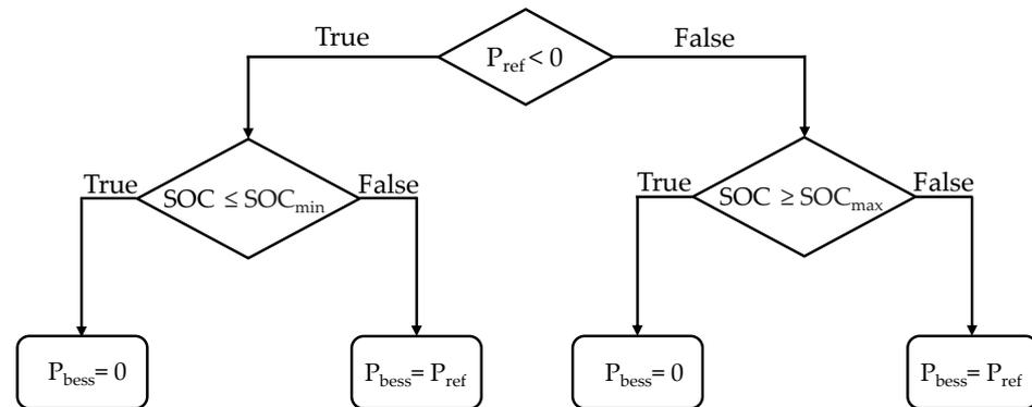
Figure 7. Flowchart for Power Smoothing control.
