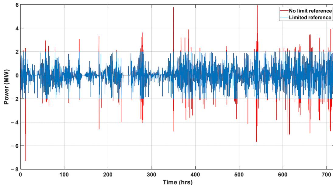
Figure 12. Comparison between ideal reference power and limited reference power.
