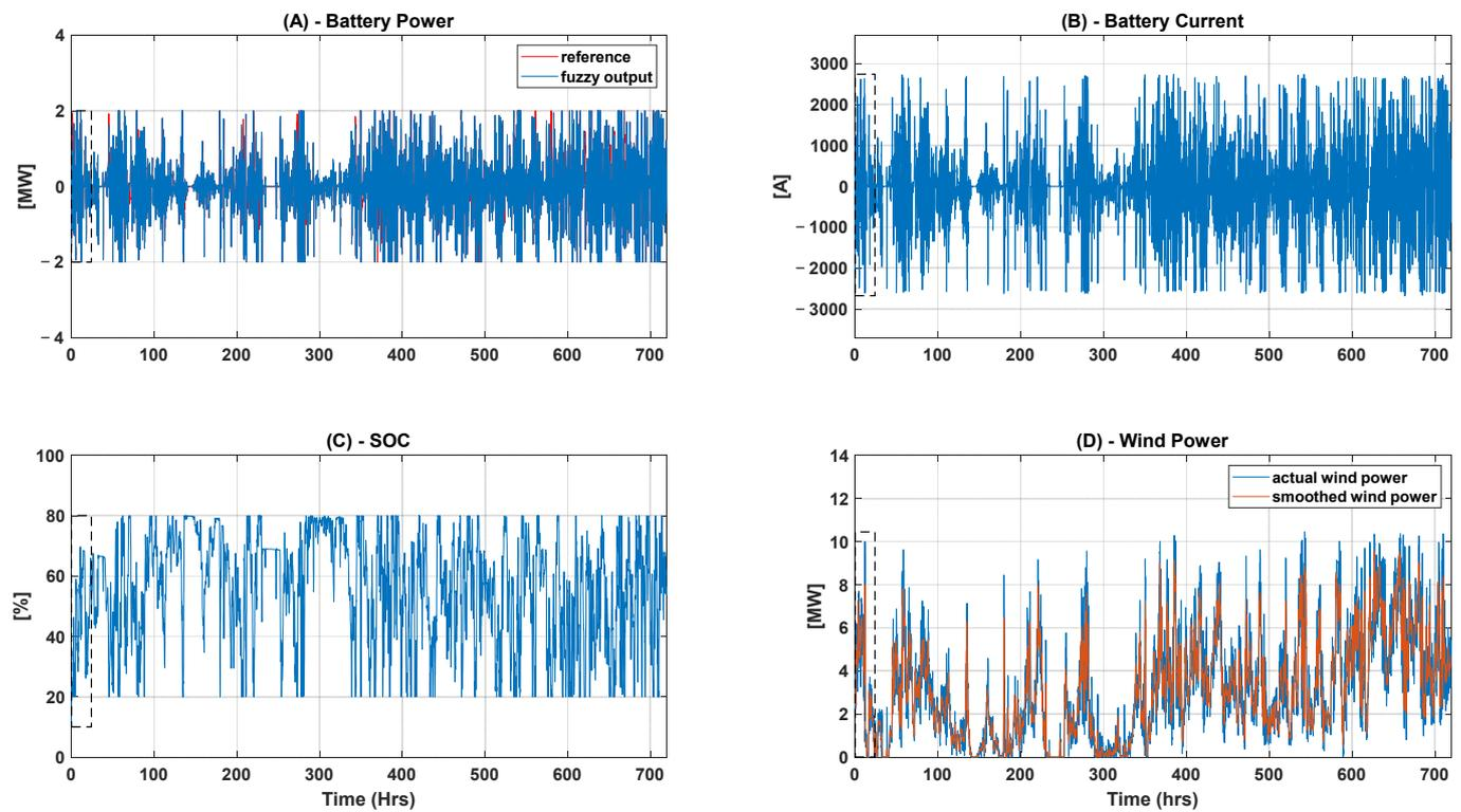
Figure 14. Simulation results for 10% initial SOC for one month. (A) Battery Power; dashed line highlight refers to Figure 13A, (B) Battery Current; dashed line highlight refers to Figure 13B, (C) SOC; dashed line highlight refers to Figure 13C, (D) Smoothed wind power; dashed line highlight refers to Figure 13D.
