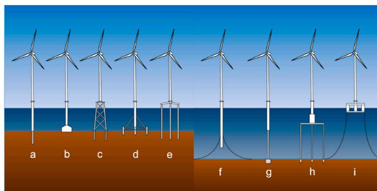
**Figure 1.** Types of OWT platforms: (a) monopile, (b) gravity-based platform, (c) jacket, (d) tripod, (e) tripole, (f) spar, (g,h) tension-legged platform, and (i) semi-submersible. Reproduced from [8], with permission from Elsevier, 2024.
