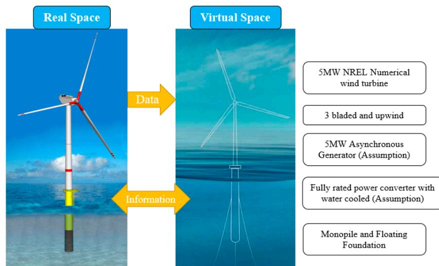
**Figure 4.** DT of a 5 MW Wind turbine with a fully rated power converter for floating applications [78,81] (completely redrawn by the authors; permission is not required).
