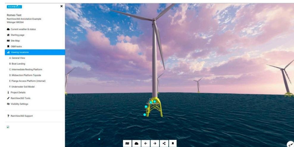
**Figure 9.** Demonstration of the DT visualisation tool RamView360 in the ROMEO project (Horizon 2020) [104] (from a public report; permission is not required).
