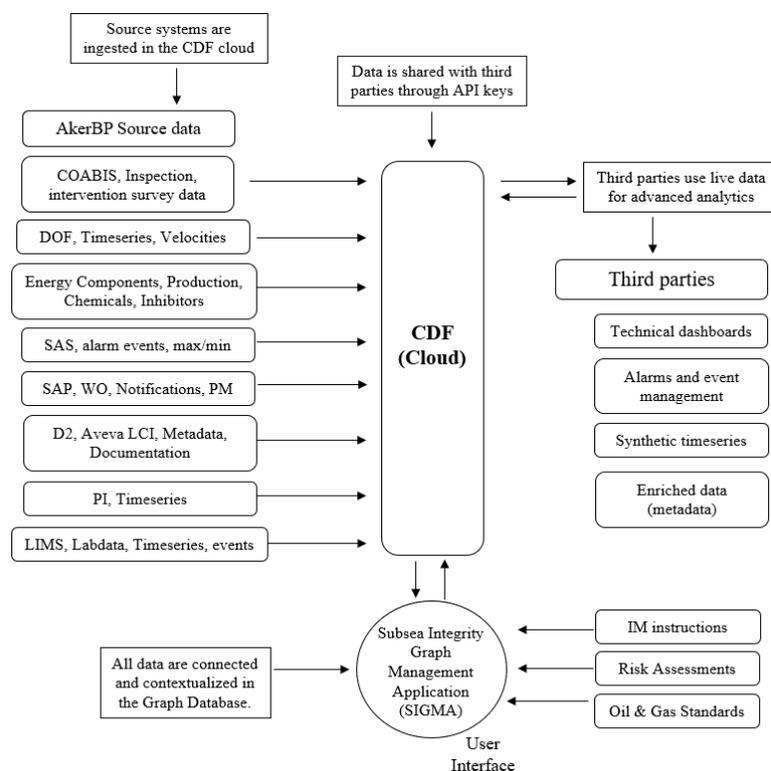
**Figure 5.** Aker BP's architecture and data flow for facilitating contextual data assessment within SIGMA for the presentation of technical conditions and risks [82] (completely redrawn by the authors; permission is not required).
