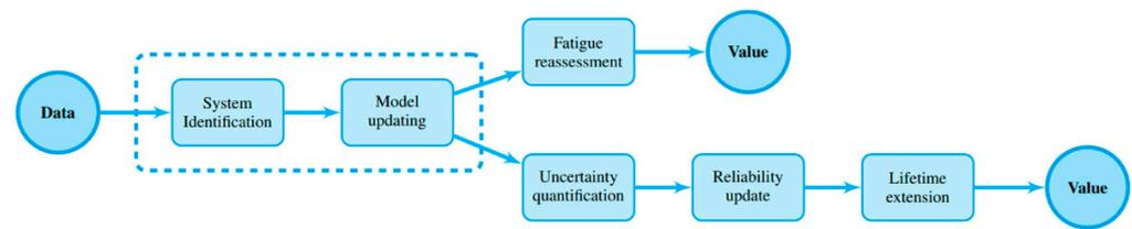
**Figure 10.** Application of a DT for lifetime extension of OWTs. Reproduced from [108], with permission from Elsevier, 2024.
