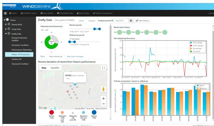
**Figure 8.** Interface of WindGemini 'Pattern of Production' module for DTs for wind turbines developed by DNV [103] (from a public report; permission is not required).
