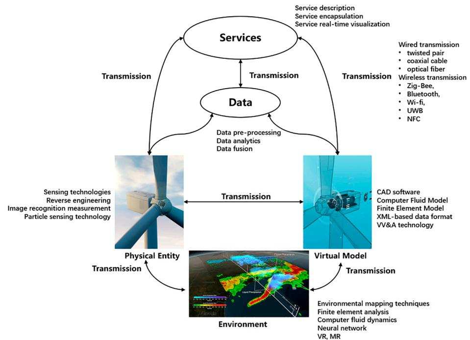
**Figure 3.** DT of a wind turbine with a variety of enabling technologies being implemented [80] (from an open-accessed journal article; permission is not required).
