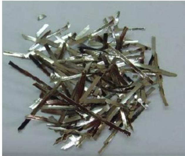
**Figure 2.** The dual-phase composite magnetic material ribbons prepared by melt-spinning method.
