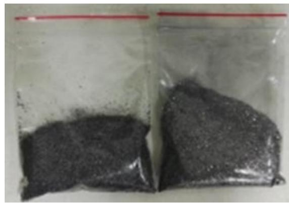
**Figure 7.** Comparison of magnetic powder with binder and without binder.
