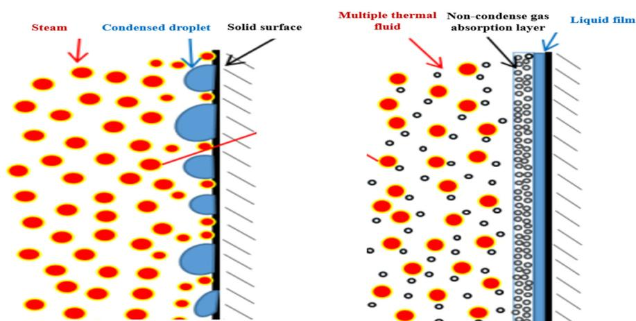
**Figure 3.** Comparison of steam stimulation with MTF stimulation in steam condensation.
