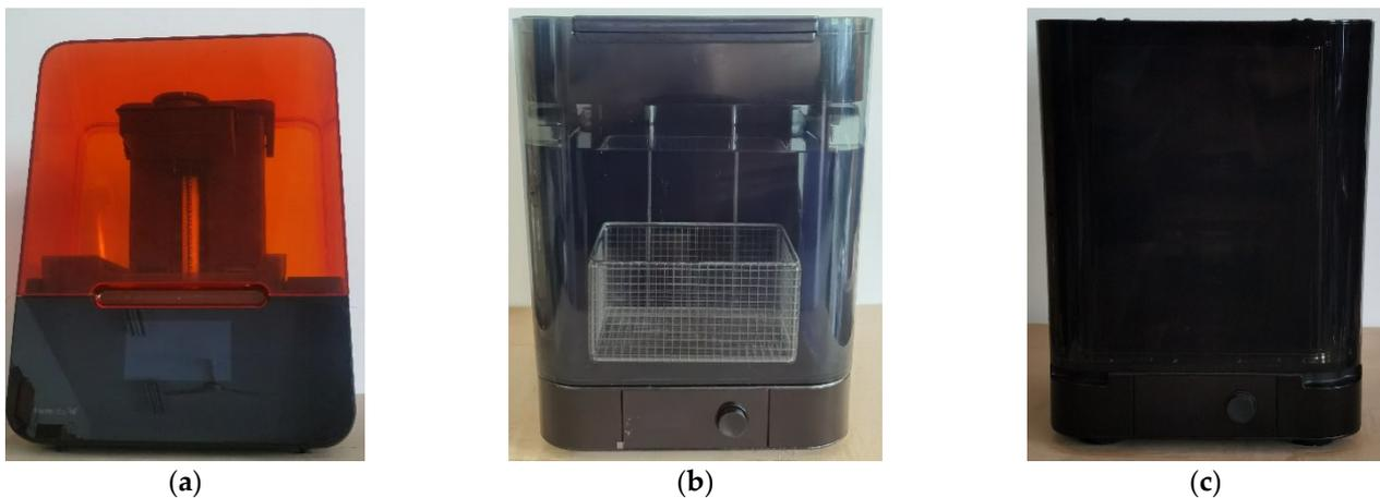
**Figure 1.** The apparatus for the material preparation. (a) Form3 low-force stereolithography 3D printer; (b) FormlabsForm wash; (c) FormlabsForm cure.
