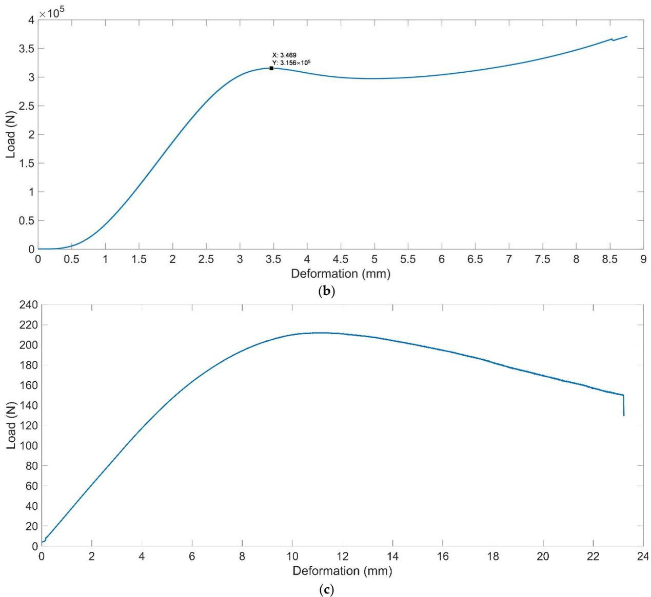
**Figure 6.** Cross-sectional experimental results of the mechanical properties of the prepared resin samples. (a) The tensile strength; (b) the compressive strength; (c) the flexural modulus.
