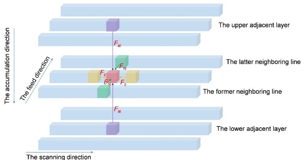
**Figure 7.** The force analysis for a single microparticle in the SLA.
