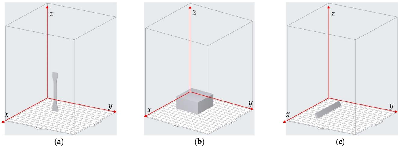
**Figure 9.** The printing orientations for the worst single mechanical property in Preform software. (a) The printing orientation for the worst tensile strength  $\sigma_b$ ; (b) the printing orientation for the worst compressive strength  $\sigma_{bc}$ ; (c) the printing orientation for the worst flexural modulus  $E$ .
