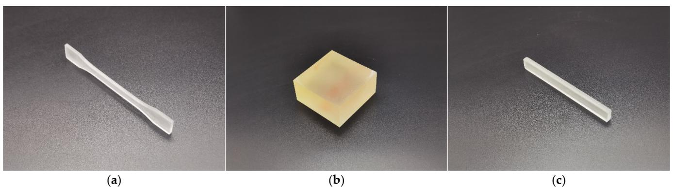
**Figure 3.** Actual photograph of the fabricated samples. (a) For the detection of tensile strength; (b) for the detection of compressive strength; (c) for the detection of flexural modulus.
