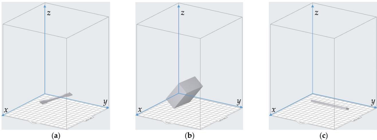
**Figure 8.** The optimal printing orientations for single mechanical properties in Preform software. (a) The optimal printing orientation for best tensile strength  $\sigma_b$ ; (b) the optimal printing orientation for best compressive strength  $\sigma_{bc}$ ; (c) the optimal printing orientation for best flexural modulus  $E$ .
