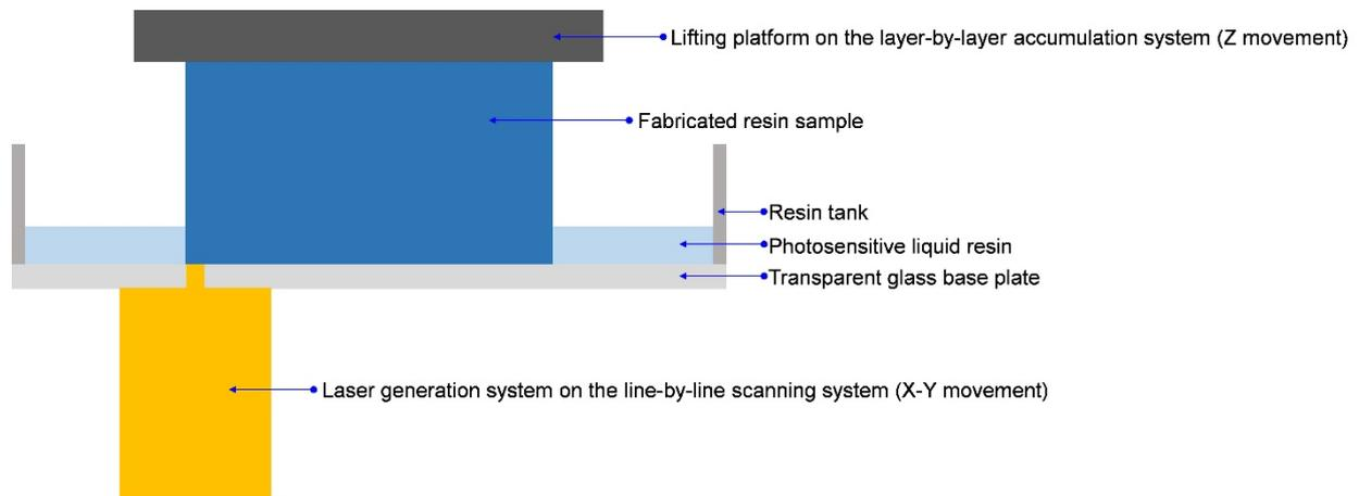
**Figure 2.** Schematic diagram of the fabrication process in the SLA.
