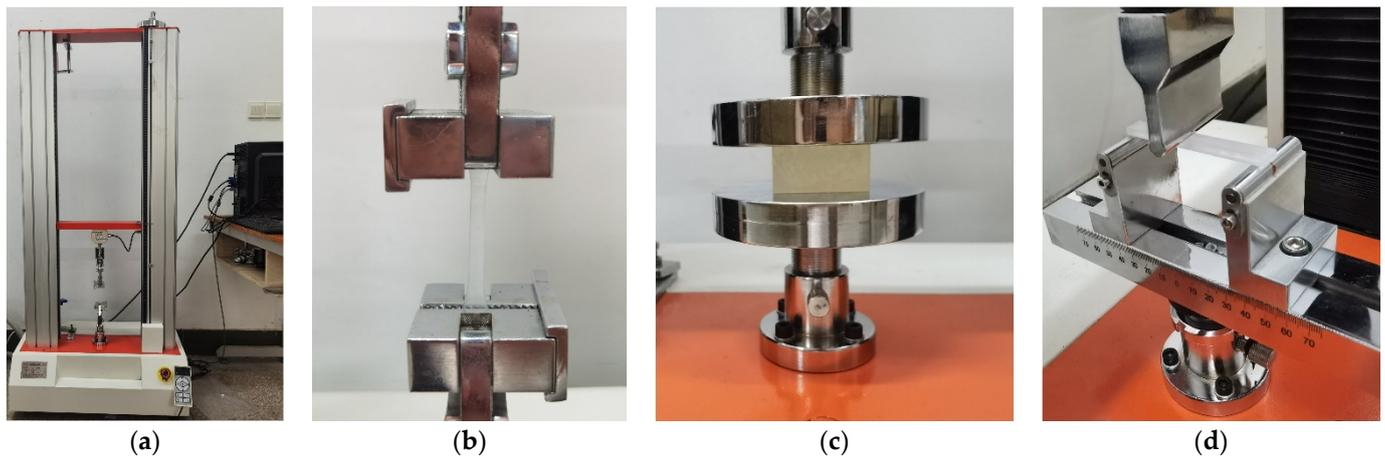
**Figure 5.** The detection of mechanical properties. (a) The universal testing machine; (b) detection of tensile strength; (c) detection of compressive strength; (d) detection of flexural modulus.
