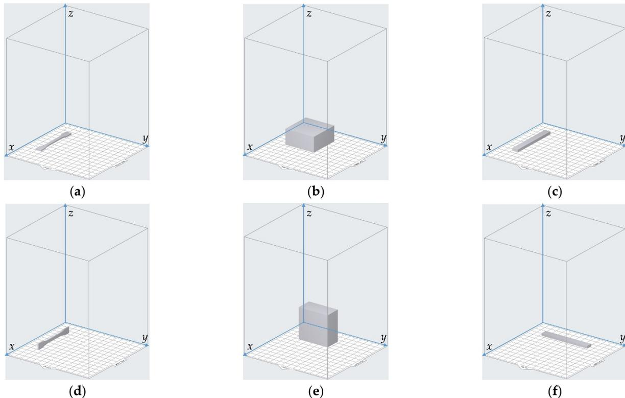
**Figure 4.** Adjustment of the printing orientations in the Preform software. (a) Default place of the sample for the detection of tensile strength; (b) default place of the sample for the detection of compressive strength; (c) default place of the sample for the detection of flexural modulus; (d) rotation  $90^{\circ}$  relative to the x-axis; (e) rotation  $90^{\circ}$  relative to the y-axis; (f) rotation  $90^{\circ}$  relative to the z-axis.
