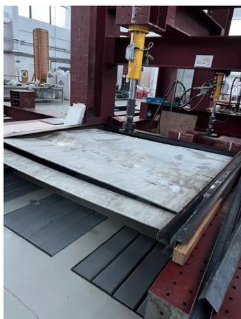
**Figure 16.** Acoustic panel mounted on a research stand.
