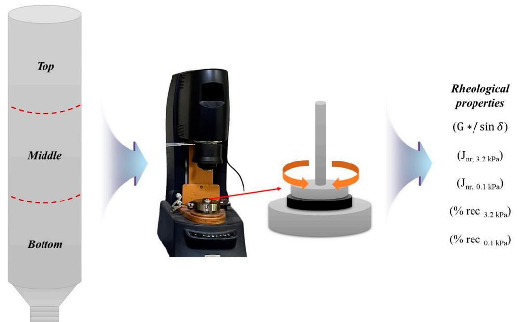
**Figure 5.** Test procedures for rheological properties.
