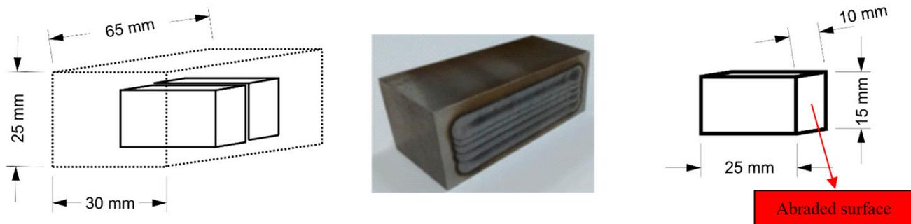
**Figure 3.** Abrasive wear test sample and the method of collecting it from the nodular cast iron casting after the surface laser remelting.
