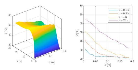
**Figure 6.** Temperature evolution in the specimen (**left**) and at discrete times (**right**) measured with fiber optic sensors.
