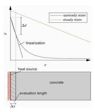
**Figure 2.** Temperature distributions in the specimen for the transient and steady-state conditions **(top)**—reduced evaluation length in the layer for an approximately linear temperature distribution (evaluation length, **bottom**).
