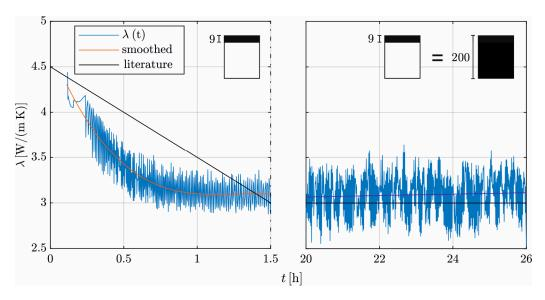
**Figure 9.** Time course of the thermal conductivity of HPC in the transition from liquid to solid with an indication of the evaluation length, compared to the literature [18].
