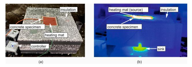
**Figure 5.** Test setup (**a**) and a thermal image during heating (**b**); in both photos, the upper insulation is removed.
