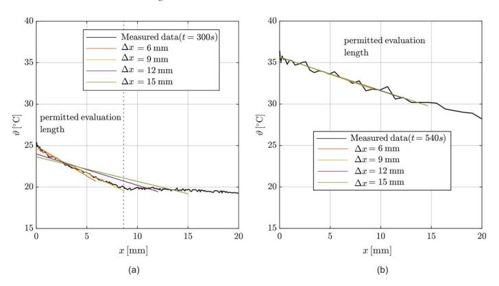
**Figure 10.** Temperature distribution in the specimen recorded by DFOS at t = 300 s (a) and t = 540 s (b) with linearized temperature gradients for different evaluation lengths  $\Delta x$ .
