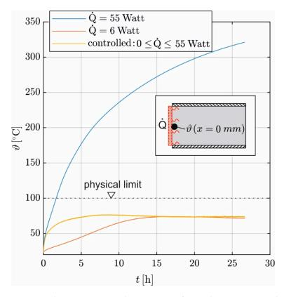
**Figure 13.** The temperature at the concrete surface with variations in induced heat according to the digital twin (Section 2.4).
