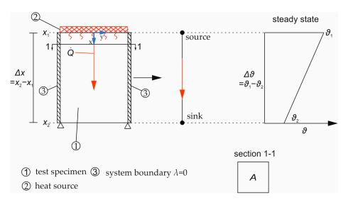
**Figure 1.** Test principle for determination of the thermal conductivity coefficient of solid materials and others with heat transfer just through thermal conduction.
