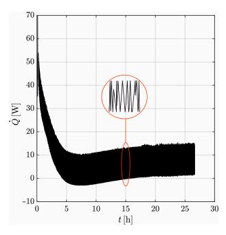
Figure 7. Heat flux over time recorded with the heat flux sensor.
