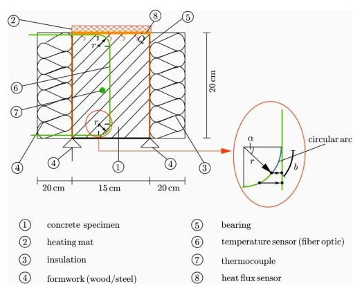
**Figure 4.** Configuration of the test rig with measurement equipment (**left**) and installation of the fiber optic sensor near the surfaces (**right**).
