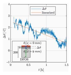
Figure 8. Time course of the linear temperature gradient on the evaluation length with linearization.
