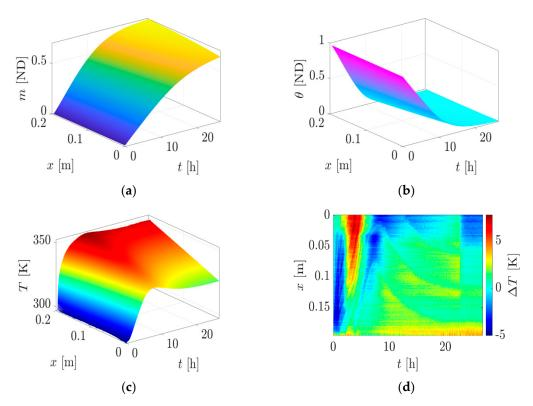
**Figure 3.** Numerical solution of Equations (9)–(11) for the parameters of Table 2 and the error between measured and numerically calculated temperature: (a) evolution of maturity; (b) evolution of moisture; (c) evolution of temperature; (d) error between the measured and numerically calculated temperature.
