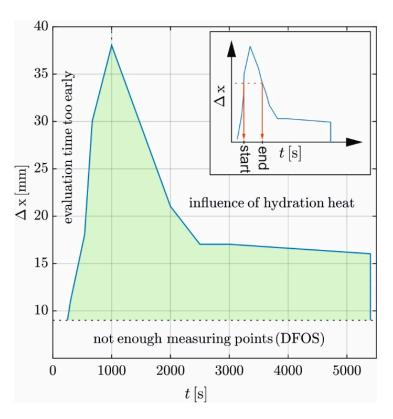
Figure 12. Relationship between evaluation length and the permissible evaluation interval.
