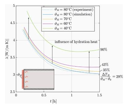
**Figure 15.** Influence of heating mat temperature  $\vartheta_M$  on the transient evolution of  $\lambda$ .
