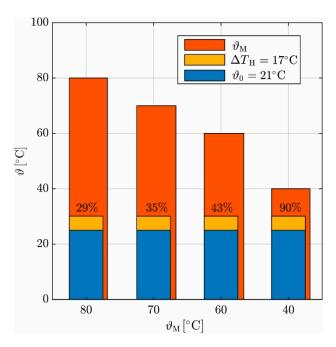
**Figure 14.** Hydration heat  $\Delta T_{\rm H}$  in relation to the externally supplied temperature  $\theta_{\rm M}$  minus the ambient temperature  $\theta_{\rm 0}$ .
