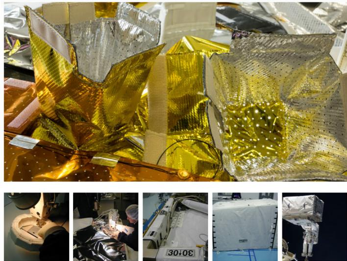
**Figure 15.** Multilayer insulation (MLI) blankets for passive thermal control in aerospace applications [130].
