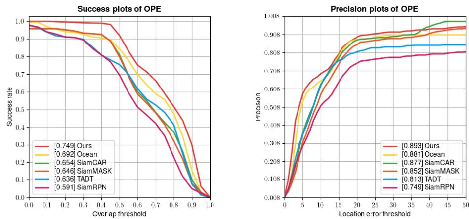
**Figure 7.** Success and precision plots on the self-built actual inspection dataset.
