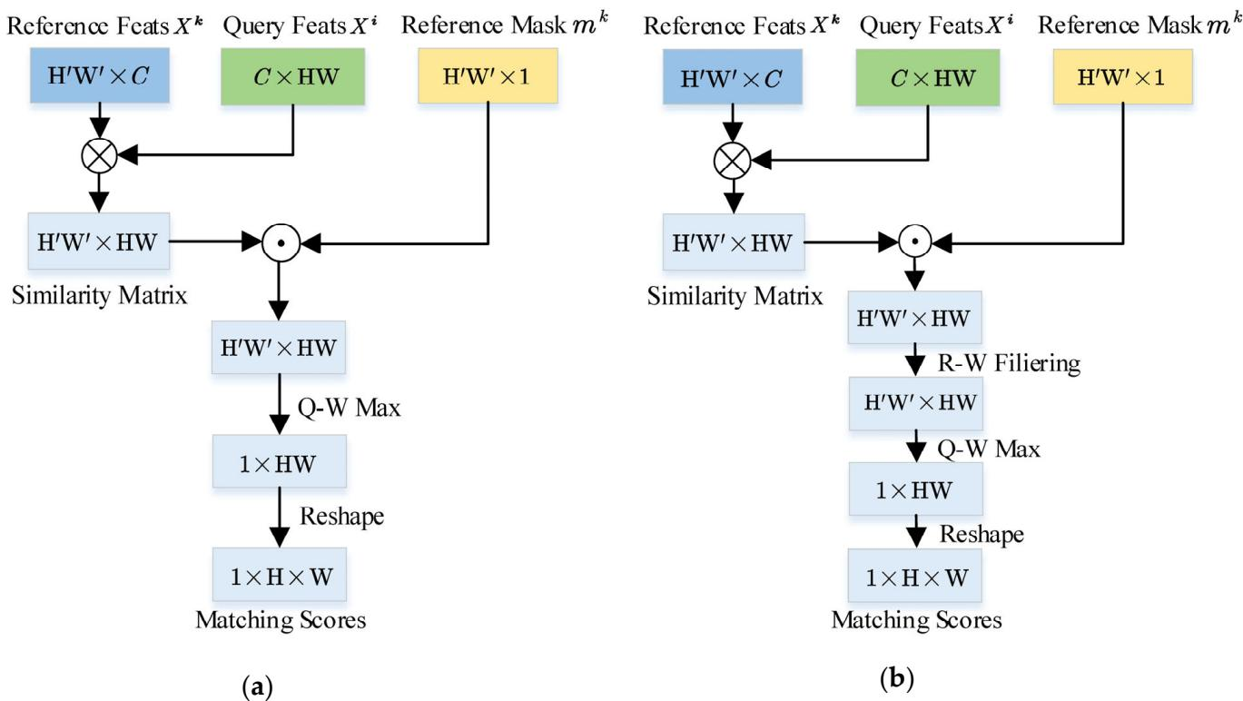
**Figure 1.** Pipelines of (a) surjective matching method and (b) bijective matching method.
