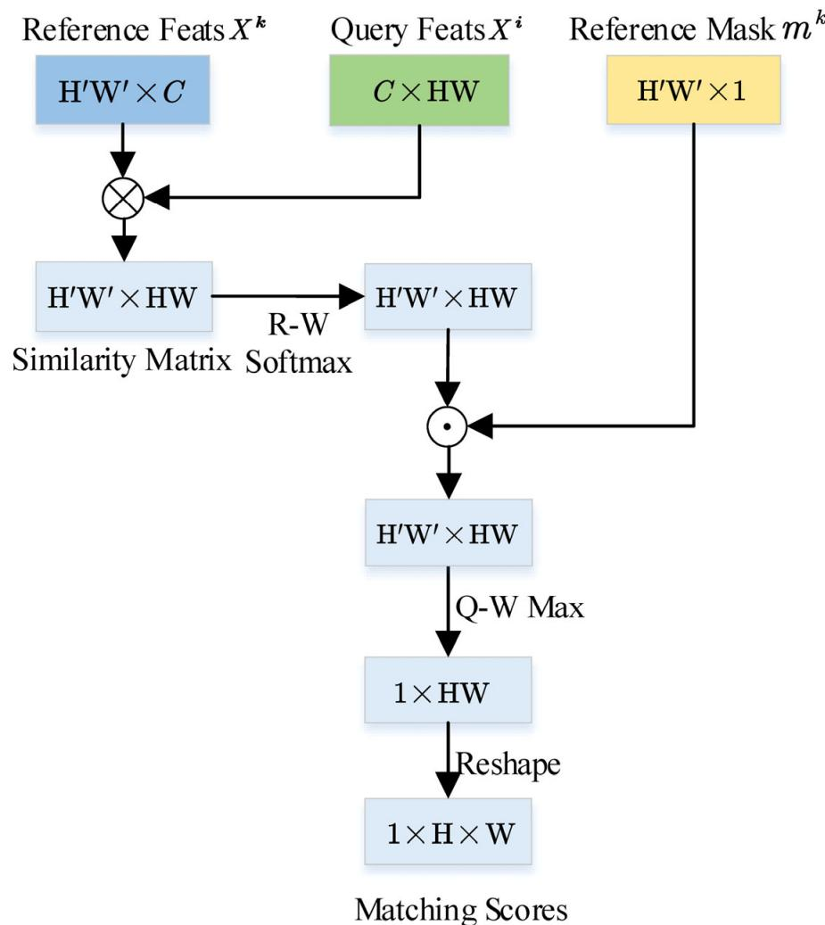
**Figure 2.** Pipelines of the equalized memory matching method.
