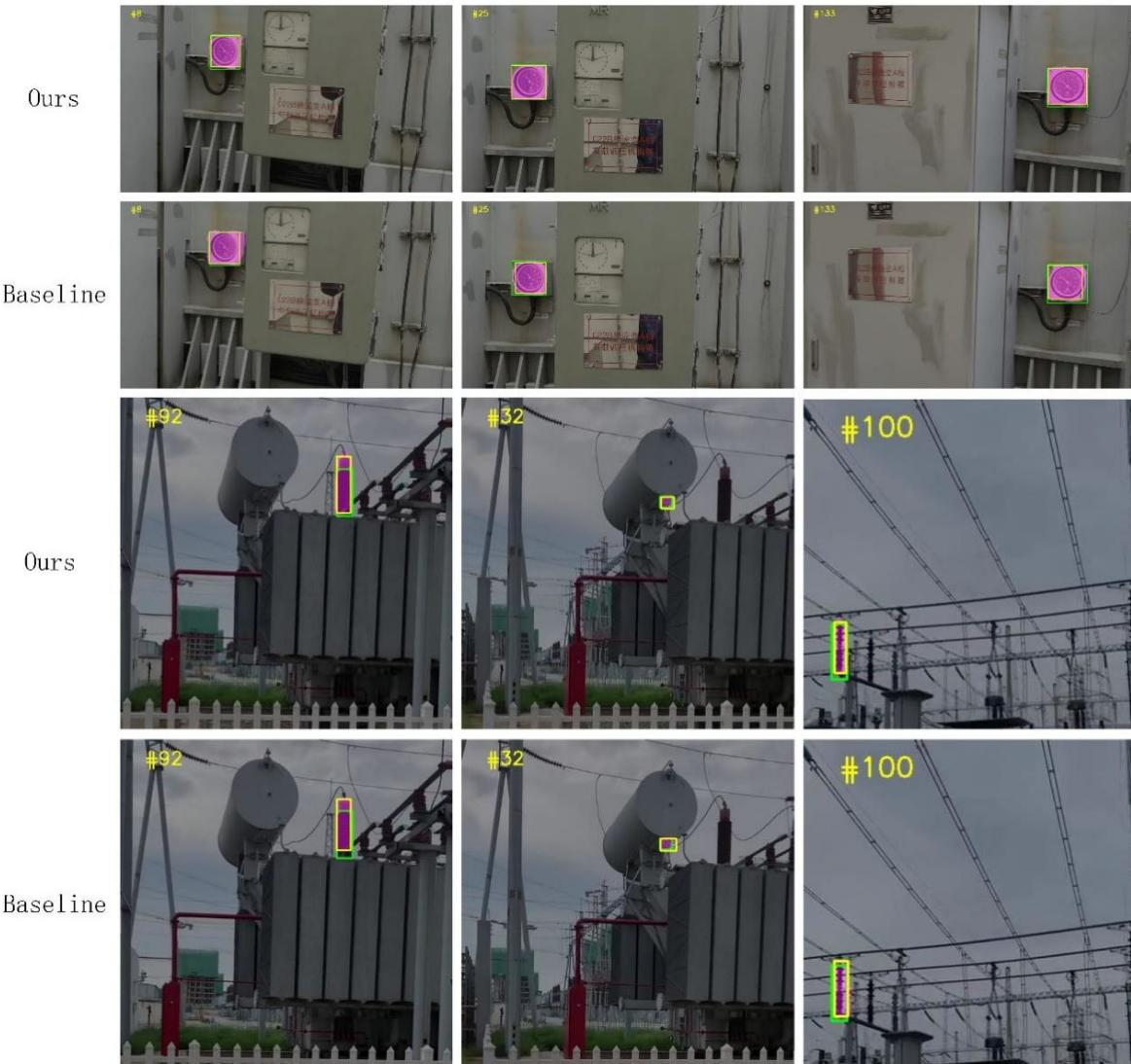
**Figure 8.** Segmentation and tracking results of our method and baseline on real inspection scene videos. The green bounding box is the ground truth, and the segmentation and tracking results are shown with the pink mask and the yellow bounding box.
