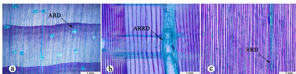
Figure 5. Microanatomical structure of *P. kesiya* var. *langbianensis*. (a) Cross-section. (b) Radial section. (c) Tangential section. ARD, Axial Resin Duct; ARRD, Axial and Radial Resin Duct Junction; RRD, Radial Resin Duct.
