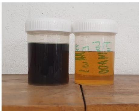
**Figure 7.** Sanitary landfill leachate before (left) and after (right) treatment with Mg/SS electrodes, at 400 mV, for 1 h.
