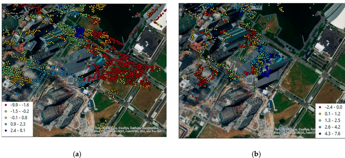
Figure 4. Geolocation of the Persistent Scatterers: (a) original position, (b) corrected position. Displacement rates in  $\text{mm}\cdot\text{yr}^{-1}$ .
