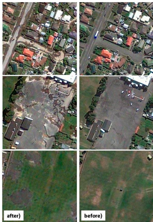
**Figure 4.** Satellite imagery before (14 February, 2011) and after (23 February, 2011) the Christchurch earthquake. Liquefied materials on the ground can be seen. Images from Google Earth. Note that these imageries are selected very close to the earthquake event date for only sake of showing the meaning of earthquake-induced liquefaction. These imageries are not use in this study for classification as they do not have any spectral information associated with them.
