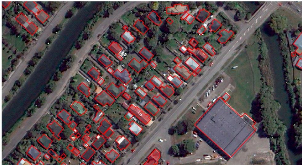
**Figure 10.** A portion of the building footprint geospatial layer used as prior knowledge to mask out roof class.
