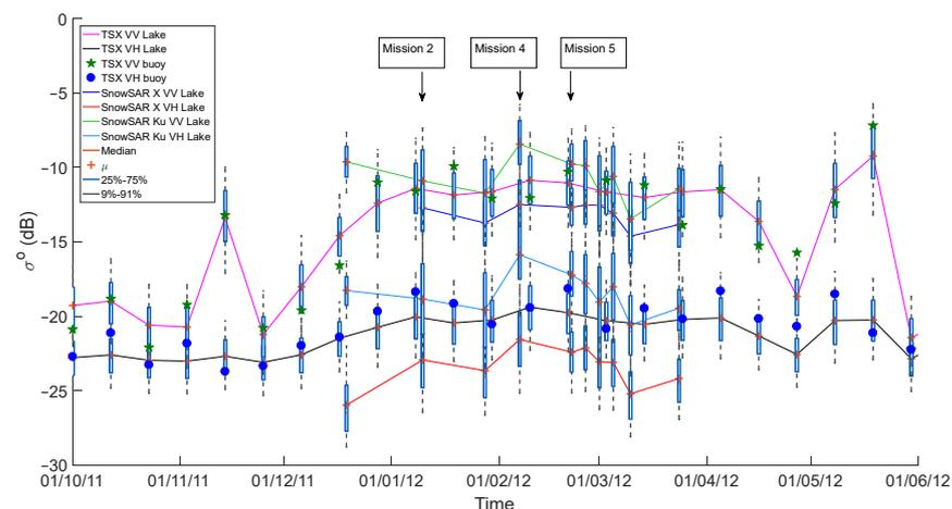
**Figure 7.** Time series of the average TSX and SnowSAR  $\sigma^0$  data at the VV- and VH-polarizations with boxplots from Lake Orajärvi in 2011–2012. In addition, the mean  $\sigma^0$  of TSX at the IMB location for VV and VH polarizations are shown as a green star and a blue circle, respectively.
