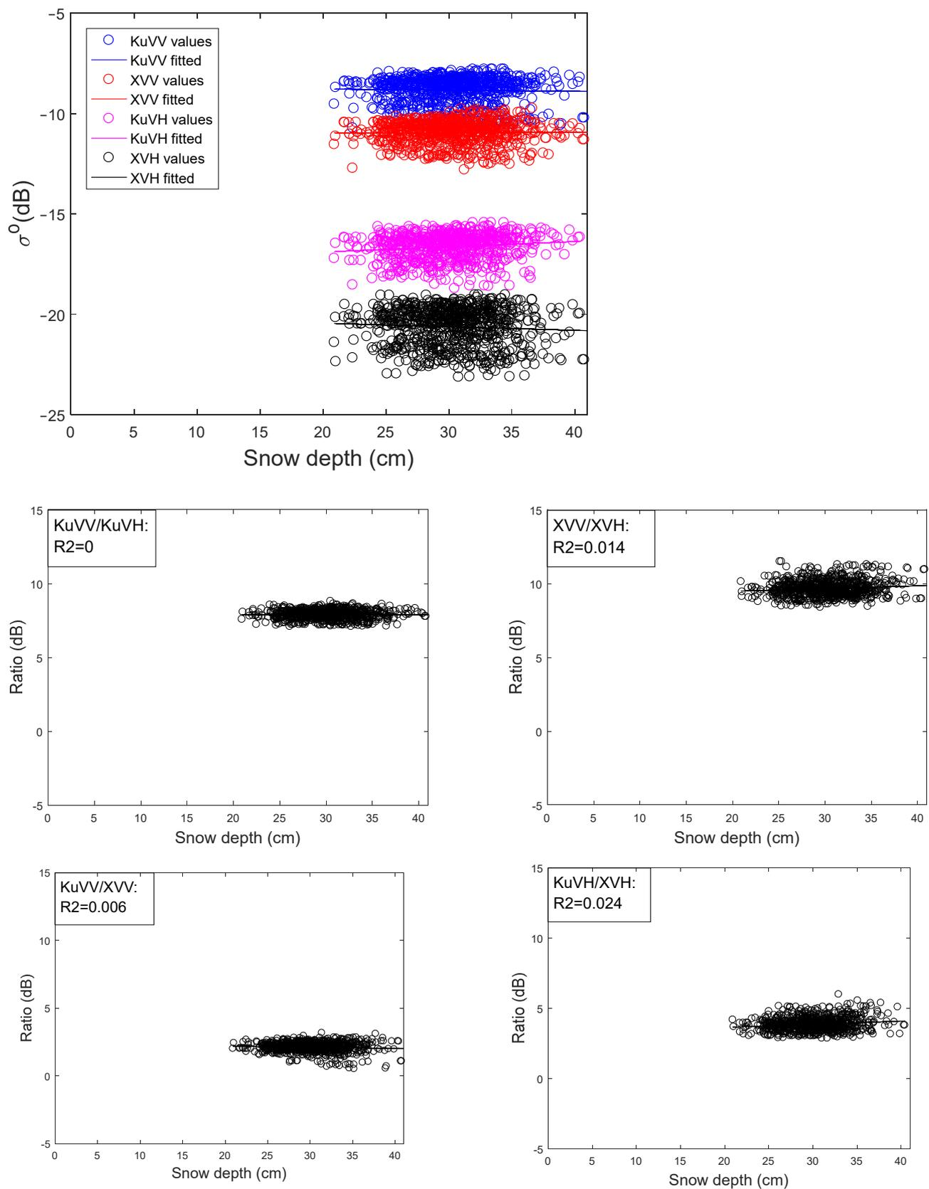
**Figure A2.** SnowSAR X- and Ku-band backscattering coefficients and their ratios as a function of snow depth on Lake Orajarvi for mission 5. The  $\sigma^0$  was scaled to the reference incidence angle of 43.8 deg for the Ku-band and 43 deg for the X-band.
