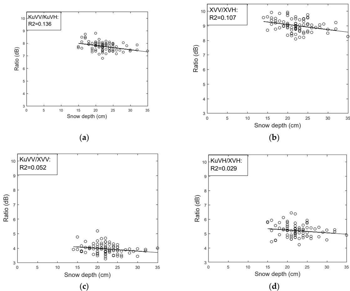
**Figure 3.** SnowSAR channel ratios as a function of snow depth on Lake Orajärvi for track1 in mission 4; (a) KuVV/KuVH, (b) XVV/XVH, (c) KuVV/XVV and (d) KuVH/XVH. Linear regression fits and coefficient of determination ( $R^2$ ) are also shown. The  $\sigma^0$  was scaled to the reference incidence angle of 43.8 deg for the Ku-band and 43 deg for the X-band.
