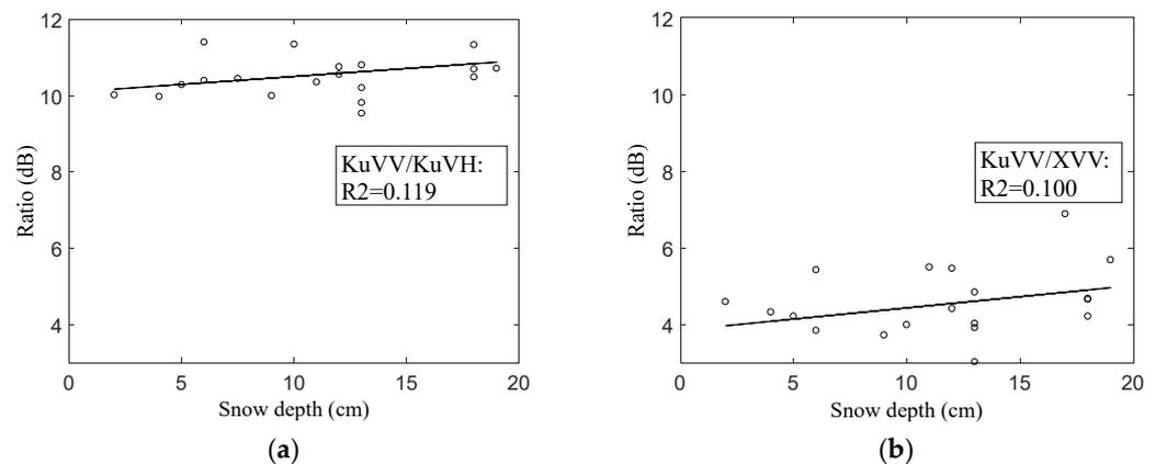
**Figure 5.** (a) Snow depth vs. SnowSAR KuVV/KuVH and (b) snow depth vs. KuVV/XVV on landfast sea ice in the Bay of Bothnia. The  $\sigma^0$  was scaled to the reference incidence angle of 43.8 deg for Ku-band and 43 deg for X-band.
