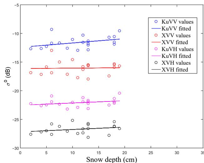
**Figure 4.** SnowSAR X- and Ku-band backscattering coefficients as a function of snow depth on landfast sea ice in the Bay of Bothnia. The  $\sigma^0$  was scaled to the reference incidence angle of 43.8 deg for Ku-band and 43 deg for X-band. The values for the coefficient of determination (R2) are listed in Table 6.
