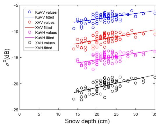
**Figure 2.** SnowSAR X- and Ku-band backscattering coefficients as a function of snow depth on Lake Orajärvi for track1 in mission 4. The  $\sigma^0$  was scaled to the reference incidence angle of 43.8 deg for the Ku-band and 43 deg for the X-band. The values for the coefficient of determination ( $R^2$ ) are listed in Table 4.
