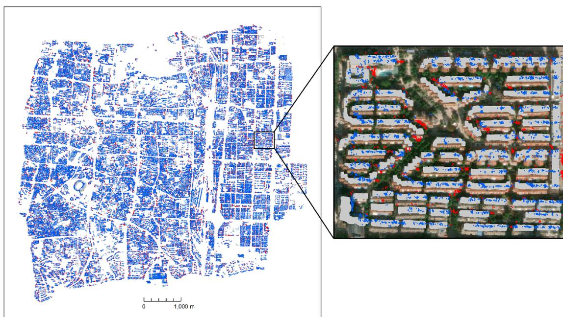
**Figure 12.** The figure shows an overlay of the results of the conventional method and new strategy. The gray areas represent the buildings, the blue dots represent the results of the traditional method, and the red dots represent the additional matching points of the new strategy.
