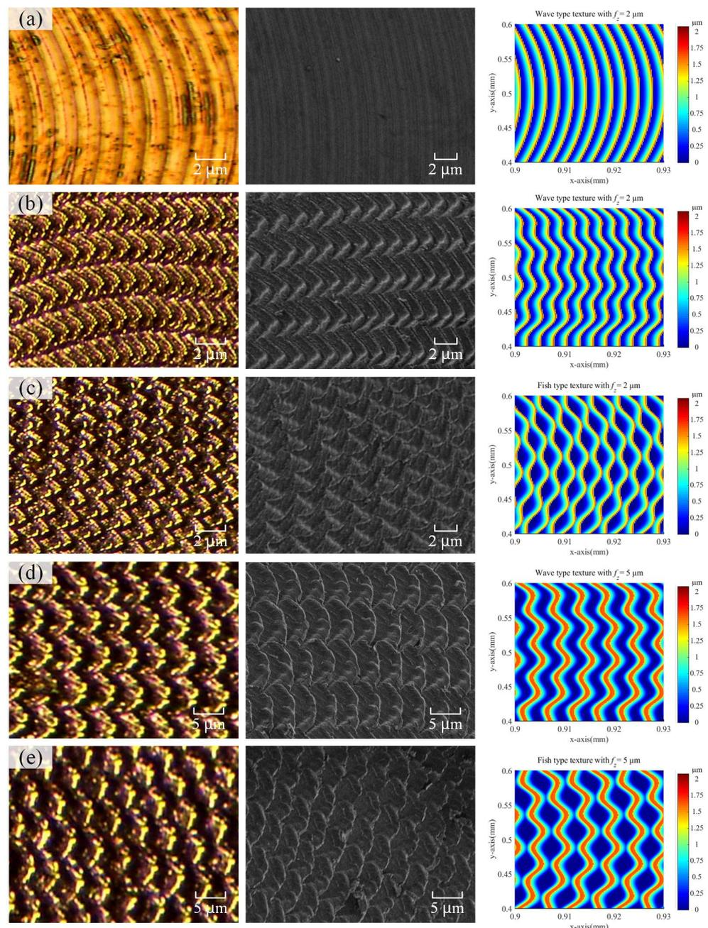
**Figure 14.** Machined surface textures observed by optical microscope and scanning electron microscope with conditions of test 1: (a); test 2: (b); test 3: (c); test 4: (d); test 5: (e).
