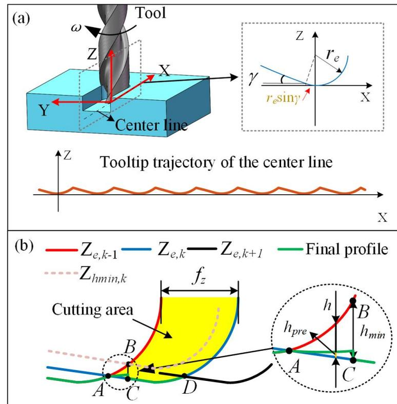
Figure 2. Micro-milling profile modeling: (a) the tooltip trajectory along the centerline, (b) machined surface profile along the centerline.
