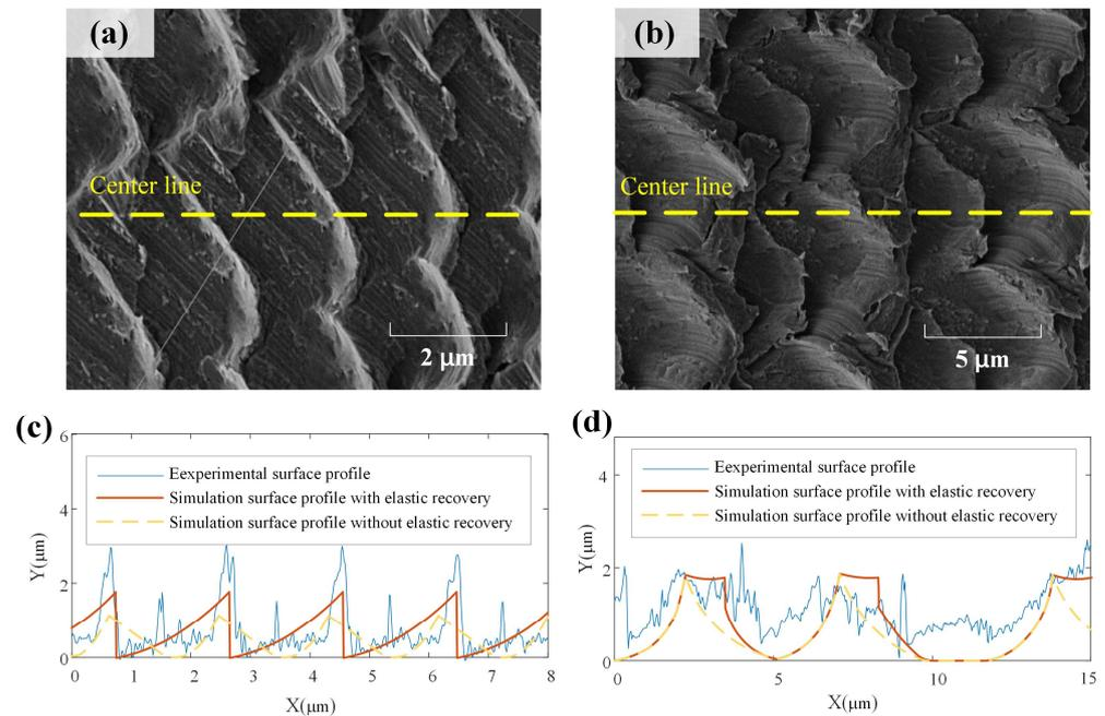
**Figure 15.** Partially enlarged surface profile: (a) surface profile of test 2, (b) surface profile of test 5, (c) center line profile of test 2, (d) center line profile of test 5.
