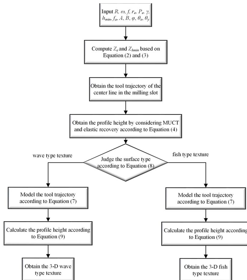
Figure 7. Flowchart to calculate the 3D surface texture.
