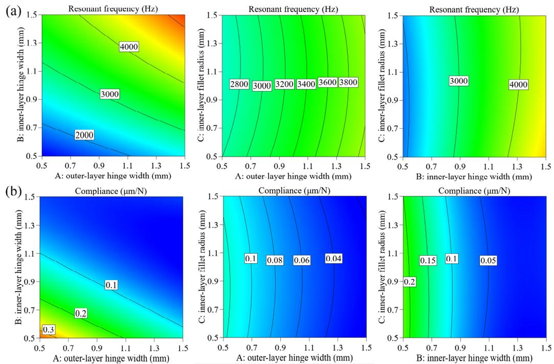
Figure 11. Contour of three parameters  $t_2, t_1, r_2$  on (a) compliance, (b) resonant frequency.
