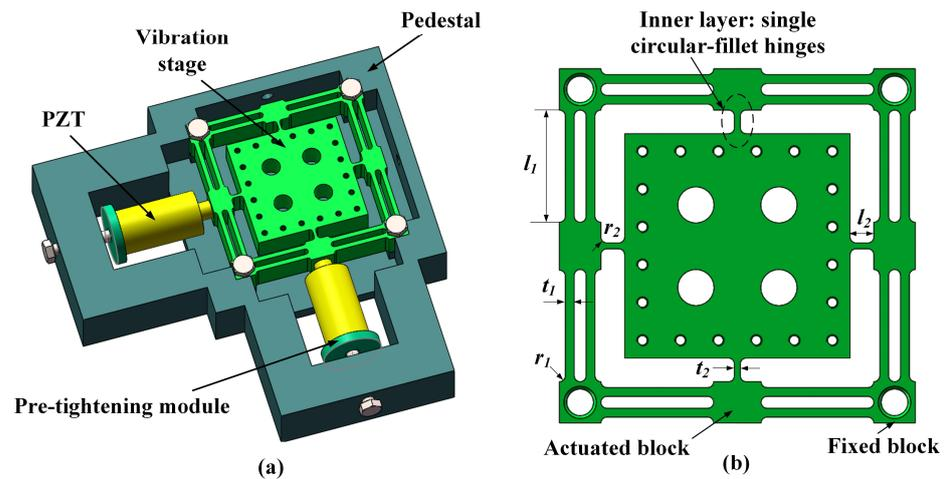
**Figure 9.** Mechanical design: (a) vibration-assisted stage, (b) flexible stage.
