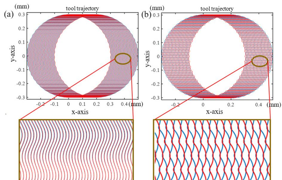
Figure 6. Two typical surface morphologies (a) wave-type trajectory, (b) fish-type tool trajectory.
