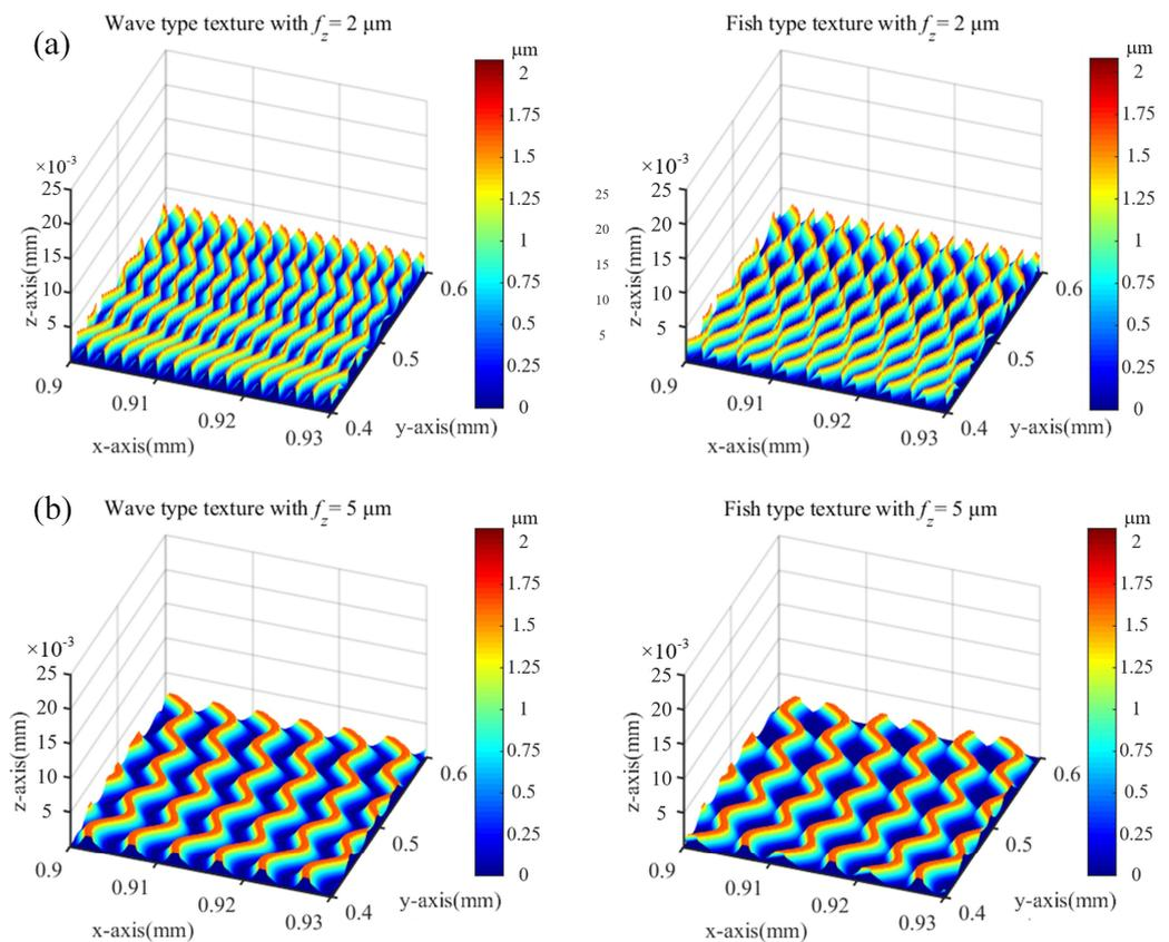
**Figure 8.** 3D surface texture with vibration-assisted under different feed per tooth (a) surface texture with  $f_z = 2 \mu\text{m}/\text{tooth}$  (b) surface texture with  $f_z = 5 \mu\text{m}/\text{tooth}$ .
