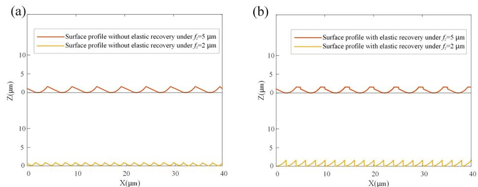
**Figure 3.** A 2D surface profile under different feeds per tooth (a) without considering elastic recovery, (b) considering elastic recovery.
