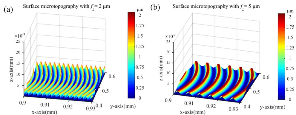
**Figure 5.** A 3D surface profile under different feeds per tooth (a)  $f_z = 2 \mu\text{m}$ , (b)  $f_z = 5 \mu\text{m}$ .
