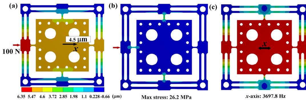
Figure 12. Finite simulation results: (a) static simulation, (b) stress distribution, (c) dynamic simulation.
