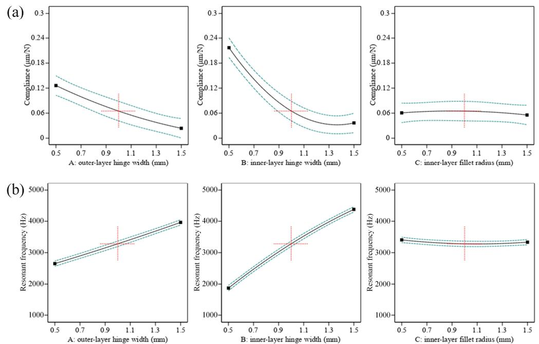
**Figure 10.** Influence of three parameters  $t_2, t_1, r_2$  on (a) compliance, (b) natural frequency.
