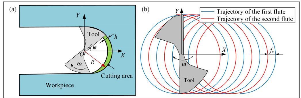
Figure 1. Micro-milling model: (a) micro end-milling operation, (b) tool trajectory.
