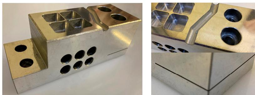
**Figure 9.** Demonstration of machining process on AyontEX 17 material, highlighting ability to machine thin-wall structures and tap holes (top-right) and EDM-processed 0.5 mm slot (left).
