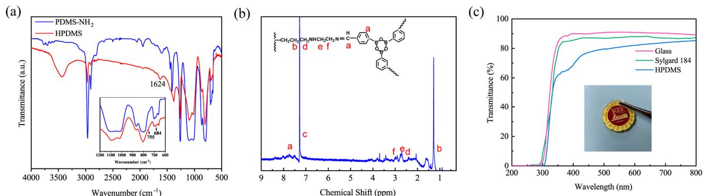
**Figure 2.** (a) FT–IR spectra of PDMS–NH<sub>2</sub> and the HPDMS elastomer. (b) <sup>1</sup>H NMR spectra of the HPDMS elastomer. (c) UV–Vis transmittance spectra of the glass slide, Sylgard 184, and HPDMS elastomer.
