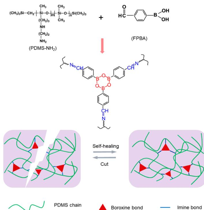
**Figure 1.** Schematic illustration of the HPDMS elastomer synthesis and the self-healing process.
