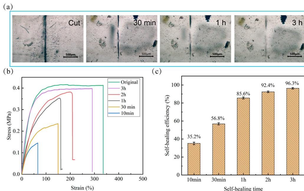
**Figure 5.** The self-healing properties of the elastomers: (a) optical microscope images, (b) stress–strain curves, and (c) self-healing efficiency of the HPDMS elastomer healed at room temperature for different times.
