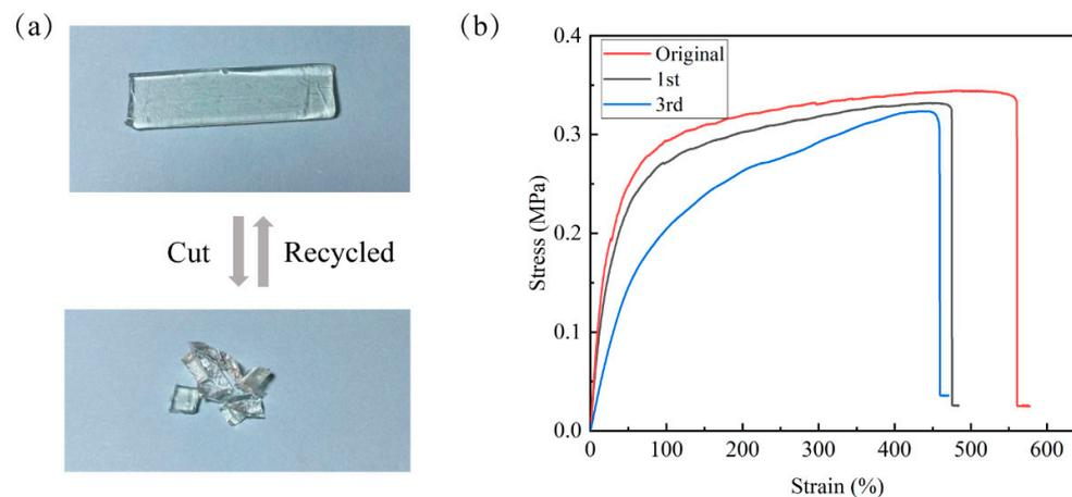
**Figure 6.** (a) Photographs of the samples were cut into small pieces and reprocessed by pressing at room temperature. (b) The stress–strain curves of the original and regenerated HPDMS elastomer.
