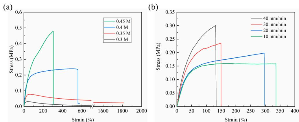
**Figure 4.** Stress–strain curves of the HPDMS elastomer (a) with different FPBA concentrations and (b) different stretching speeds.
