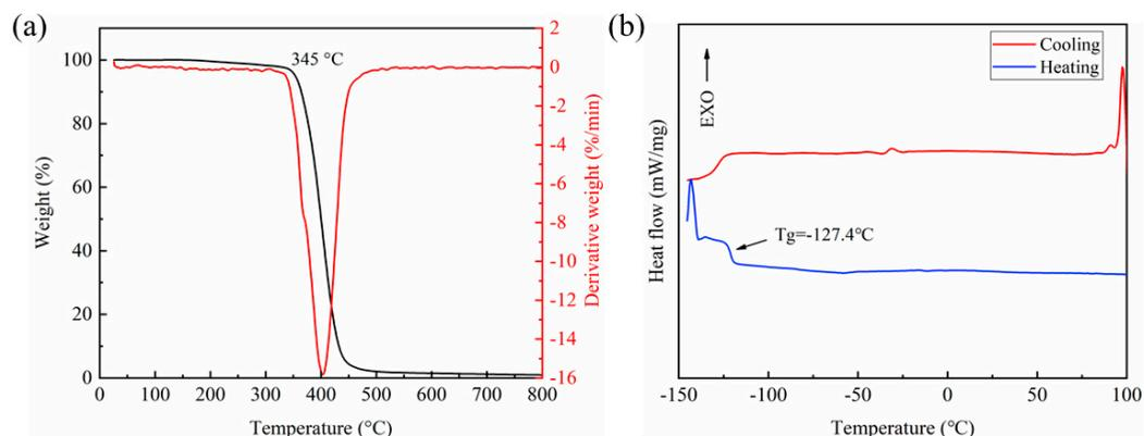
**Figure 3.** (a) TGA curves and (b) DSC traces of the HPDMS elastomer.
