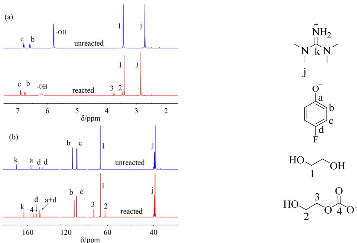
**Figure 2.** The  $^1\text{H}$  (a) and  $^{13}\text{C}$  (b) NMR spectra of [TMGH][4-F-PhO]:EG (1:3) with and without  $\text{CO}_2$ .
