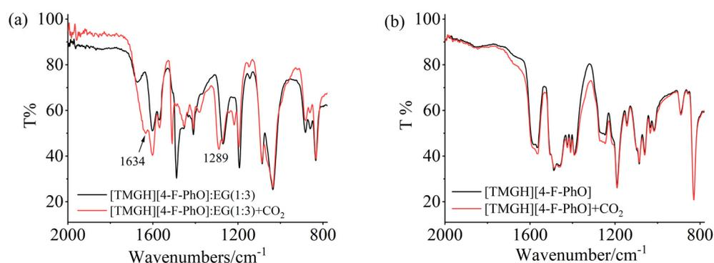
**Figure 4.** The FTIR spectra of [TMGH][4-F-PhO]:EG (1:3) (a) and [TMGH][4-F-PhO] (b) before and after absorption.
