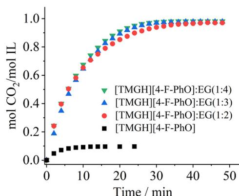
Figure 1. CO<sub>2</sub> uptake by [TMGH][4-F-PhO]-EG and [TMGH][4-F-PhO] at 25 °C and 1.0 atm.
