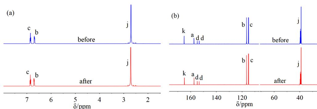
**Figure 3.** The  $^1\text{H}$  (a) and  $^{13}\text{C}$  (b) NMR spectra of [TMGH][4-F-PhO] with and without  $\text{CO}_2$ .
