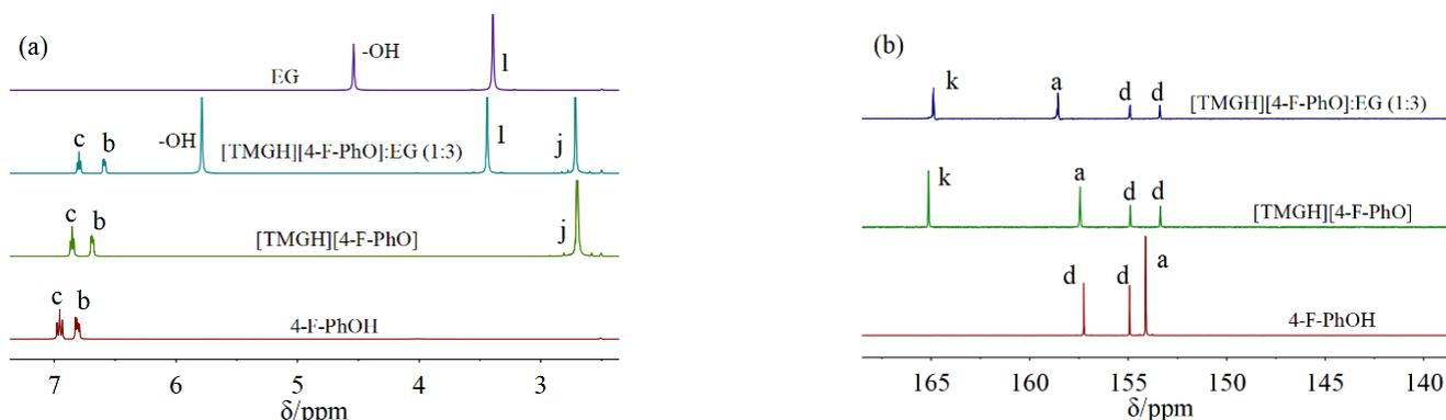
**Figure 5.** (a) The <sup>1</sup>H NMR spectra of EG, [TMGH][4-F-PhO]:EG (1:3), [TMGH][4-F-PhO], and 4-F-PhOH; (b) <sup>13</sup>C NMR spectra of [TMGH][4-F-PhO]:EG (1:3), [TMGH][4-F-PhO], and 4-F-PhOH.
