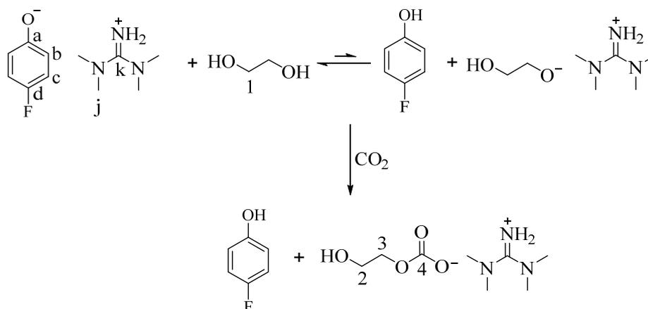
**Scheme 1.** The possible reaction mechanism between  $\text{CO}_2$  and [TMGH][4-F-PhO]-EG solvents used in this work.
