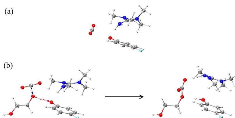
**Figure 8.** The interactions between CO<sub>2</sub> and absorbents: (a) [TMGH][4-F-PhO] + CO<sub>2</sub>; (b) [TMGH][4-F-PhO]-EG + CO<sub>2</sub>.
