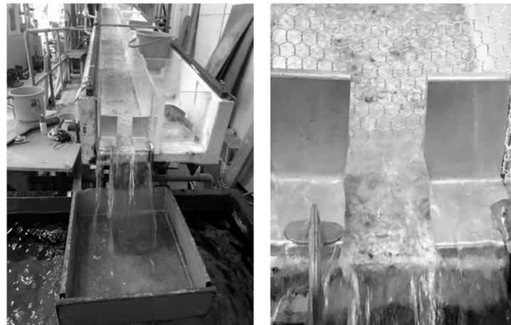
Figure 9. Photo of the permeable debris flow barrier used in the experiments.
