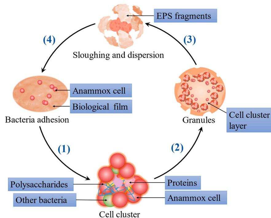
**Figure 2.** Granulation cycle mechanism. Mechanism based on EPS adhesion. (1) bacterial attachment to solid surfaces or self-aggregation; (2) production and accumulation of EPS; (3) maturation of three-dimensional structures; and (4) detachment and recolonization.
