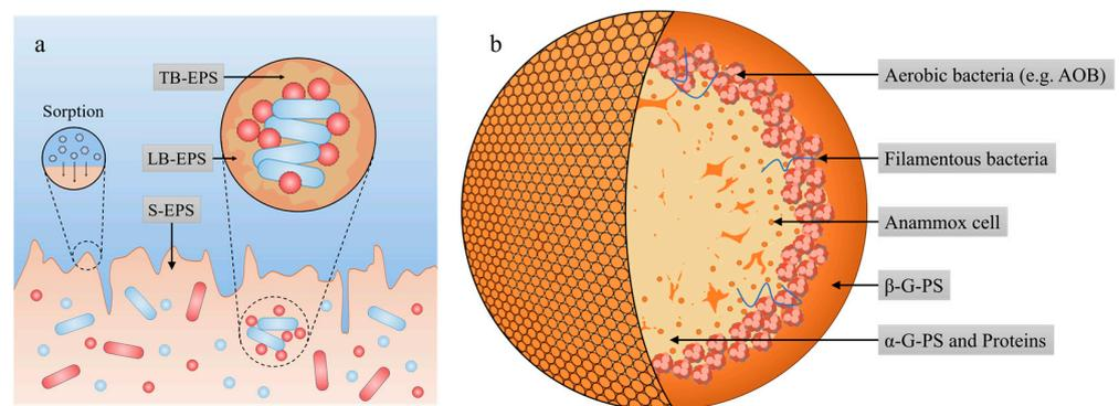
**Figure 1.** Schematic diagram of EPSs in anaerobic ammonia oxidation biofilm (a) and granular sludge (b). TB-EPS: soluble EPS; LB-EPS: loosely bound EPS; S-EPS: tightly bound EPS;  $\beta$ -G-PS:  $\beta$ -glucopyranose polysaccharides;  $\alpha$ -G-PS:  $\alpha$ -D-glucopyranose polysaccharides. Sorption: nutrients and other molecules can be trapped by sorption to EPSs.
