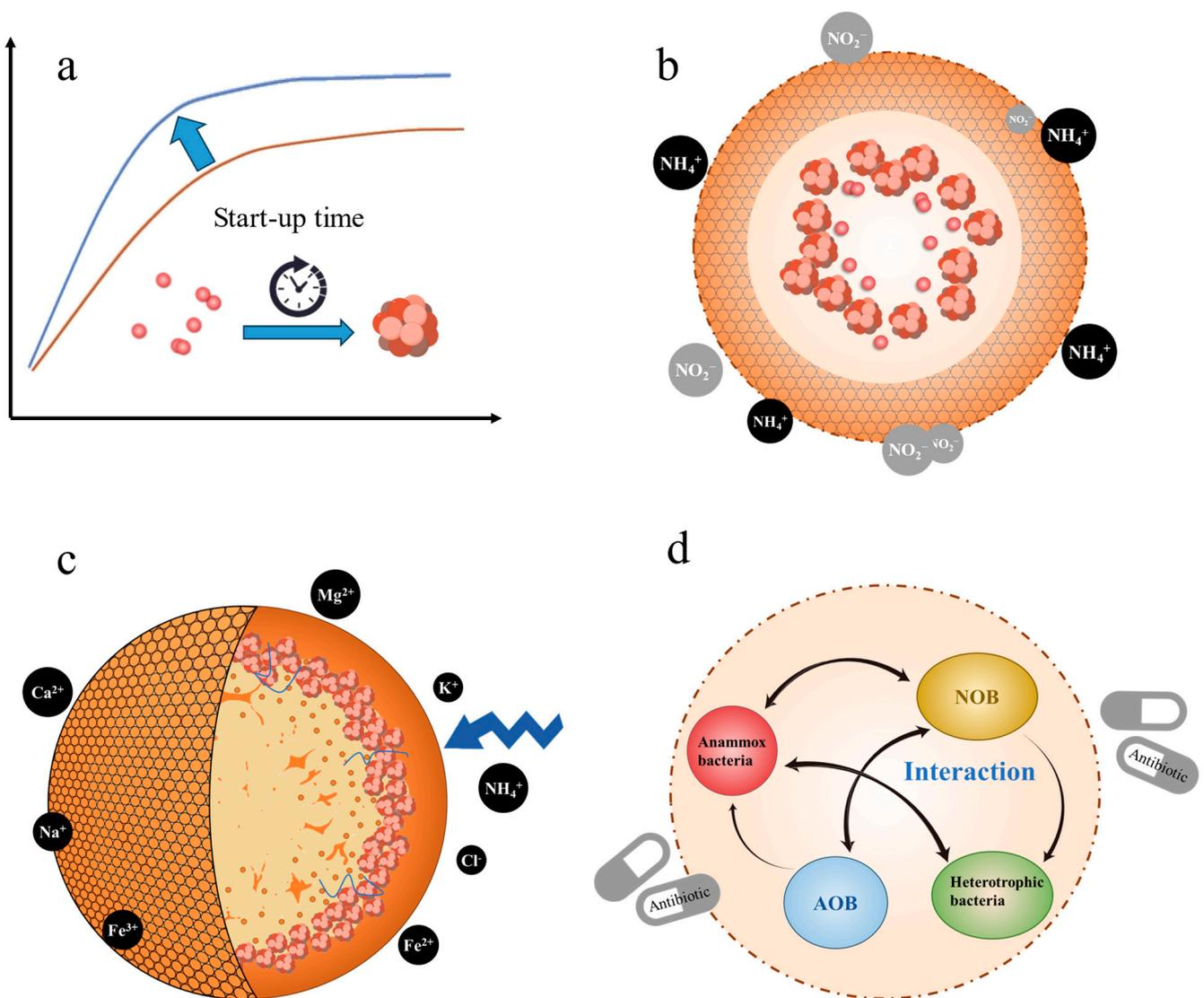
**Figure 4.** Examples of EPSs improving ANAMMOX performance. (a) fast start-up by accelerating cell aggregation; (b) wrap cells to reduce substrate penetration; (c) reduce direct contact between cells and salt ions; (d) microbial community diversity promotes recovery.
