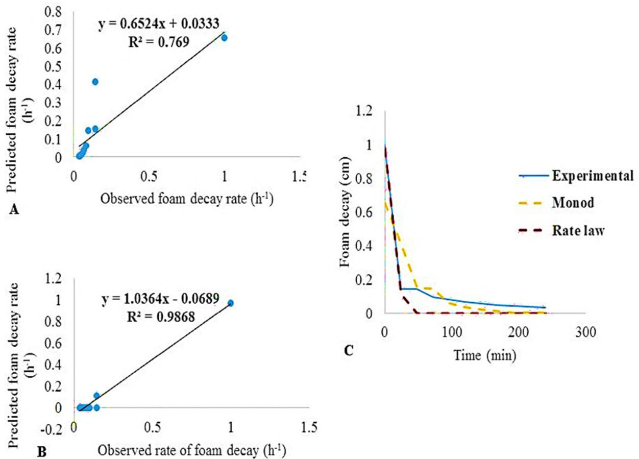
**Figure 3.** Consistency plots of (A) Monod's model, (B) the rate law, and (C) illustration of the model plots in comparison to experimental foam decay data.
