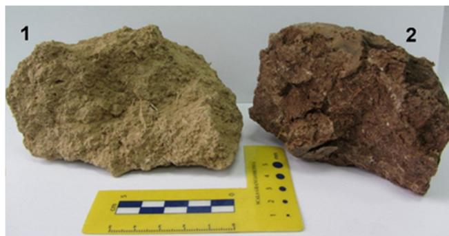
**Figure 2.** Investigated samples from Rujiste deposit: 1-light brown clay (sample 1), 2-dark brown-colored clay (sample 2).
