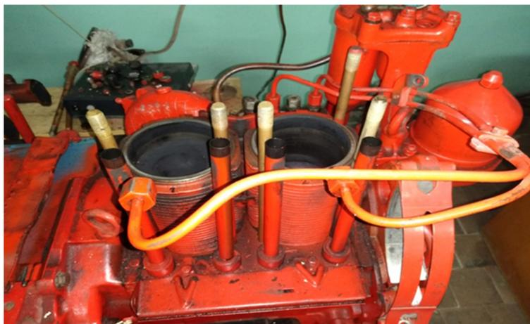
**Figure 6.** The experimental diesel engine with dismantled heads of the block.
