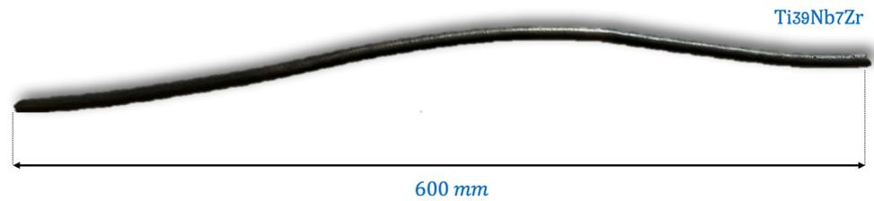
**Figure 2.** Photographic image of the Ti<sub>39</sub>Nb<sub>7</sub>Zr rod after rotary forging.
