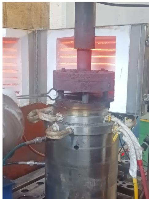
**Figure 4.** Hot-stamping-forming experiment equipment.
