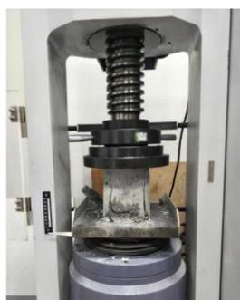
**Figure 1.** Compressive test for concrete.
