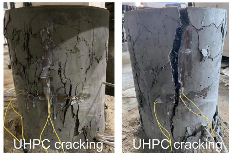
Figure 4. Z4 and Z5 failure forms.
