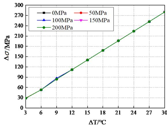
Figure 26. The variation in the stress differential with temperature under different stress levels.
