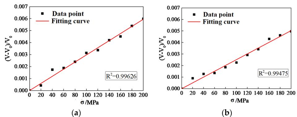
Figure 19. The relationship between the relative wave velocity and stress. (a) The relationship for A1 (b) The relationship for B1.
