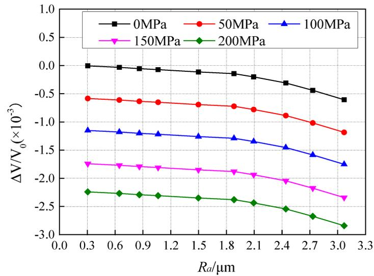
Figure 29. The variation in the relative wave velocity with  $Ra$  under different stress levels.
