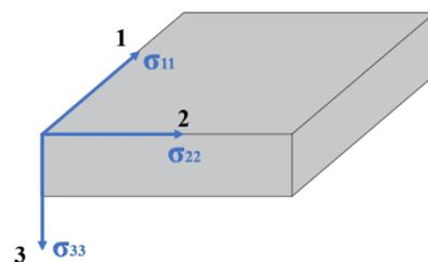
Figure 3. The direction of principal stress.
