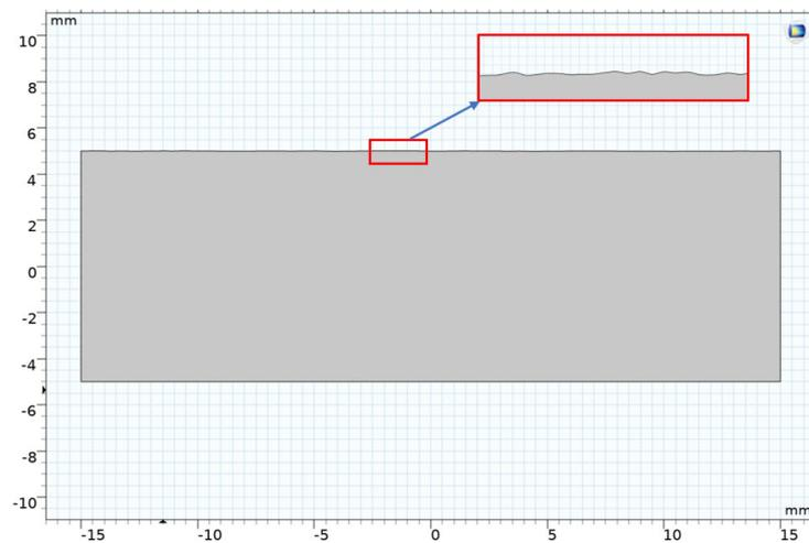
Figure 28. The FE model with a rough surface.
