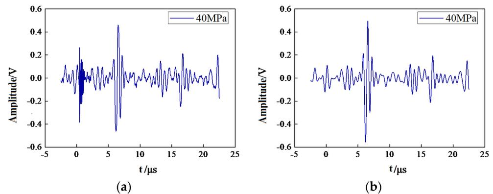
**Figure 15.** Ultrasonic time-domain signal for B1. (a) Ultrasonic time—domain signal before wavelet denoising; (b) Ultrasonic time-domain signal after wavelet denoising.
