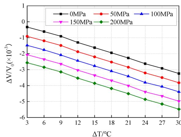
Figure 25. The variation in the relative wave velocity with temperature under different stress levels.
