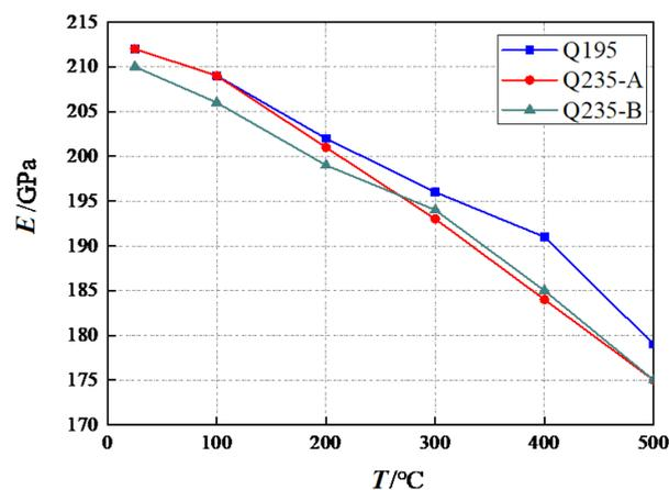
**Figure 24.** The elastic modulus at different temperatures.
