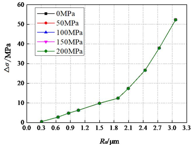
Figure 30. The variation in the stress differential with  $Ra$  under different stress levels.
