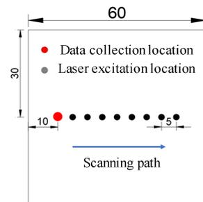
Figure 13. The scanning path of the specimen under stress-free conditions/mm.
