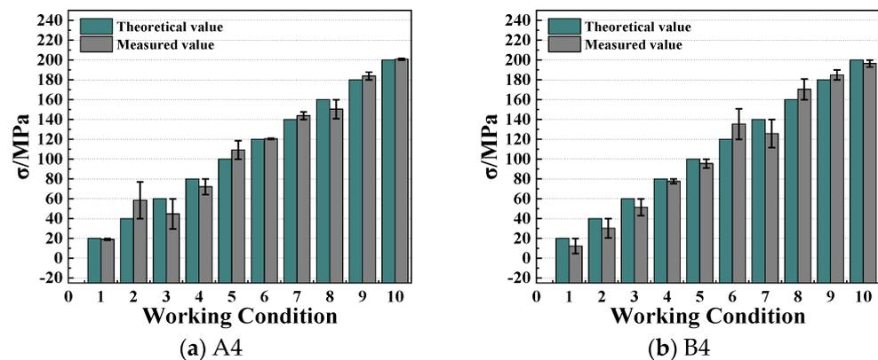
Figure 22. Stress calculation results for theoretical propagation distance at 20 mm.
