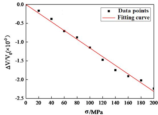
Figure 9. Relationship between the relative wave velocity of ultrasound and stress.
