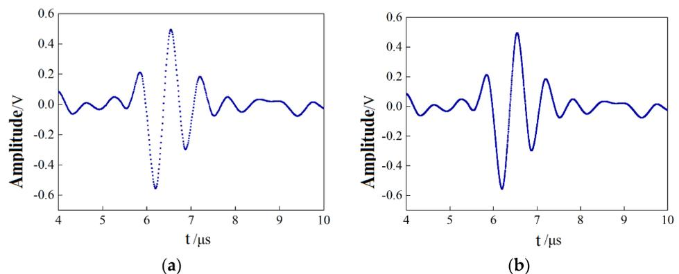
**Figure 16.** Ultrasonic time-domain signal for B1. (a) Ultrasonic time-domain signal before interpolation (b) Ultrasonic time-domain signal after interpolation.
