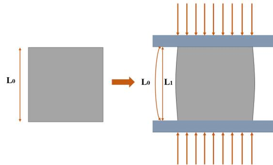
**Figure 17.** The surface changes of the specimen during the loading process.
