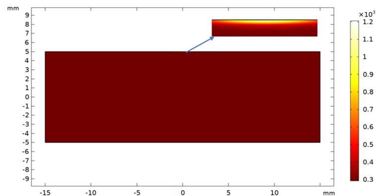
**Figure 6.** The temperature distribution of the whole field when  $t$  is 70 ns.
