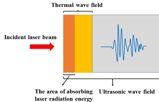
**Figure 2.** The principle of the excitation with laser ultrasonics.
