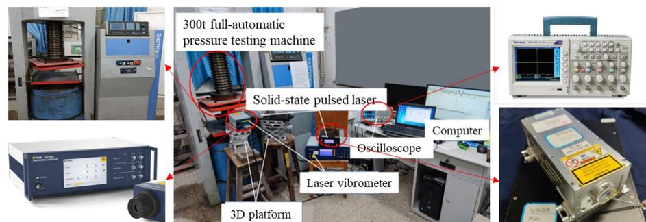
**Figure 12.** The laser ultrasonic testing system.
