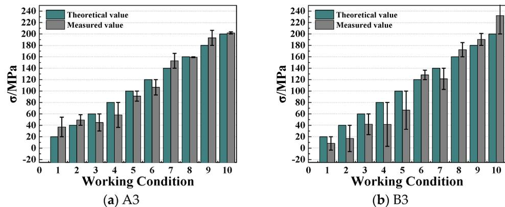
Figure 21. Stress calculation results for theoretical propagation distance at 10 mm.
