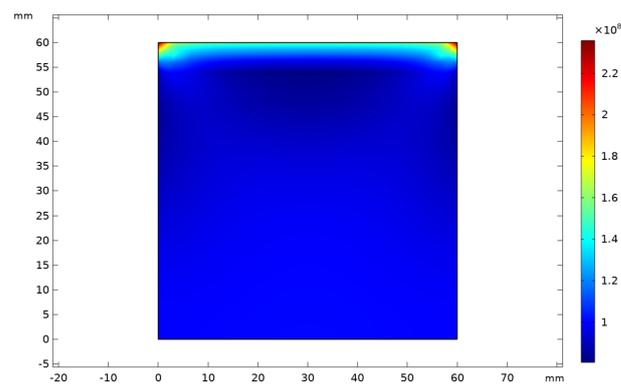
**Figure 11.** The distribution of stress on the side surface under uniaxial stress.
