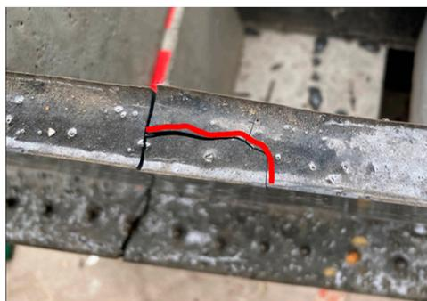
Figure 6. Interlayer cracks.
