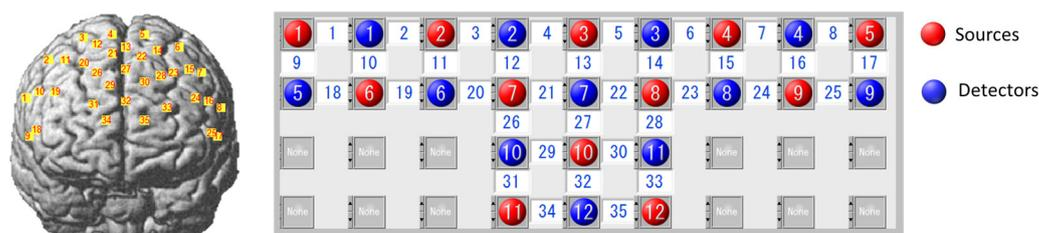
**Figure 1.** Channel layout and position of light sources and detectors.
